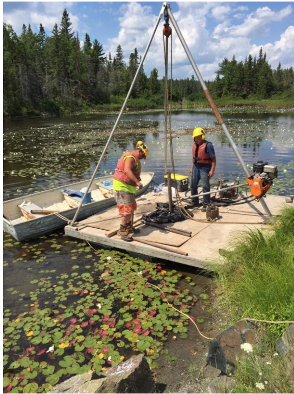
Photograph 5: Drilling Borehole WL-04 with Portable Rig on Barge
