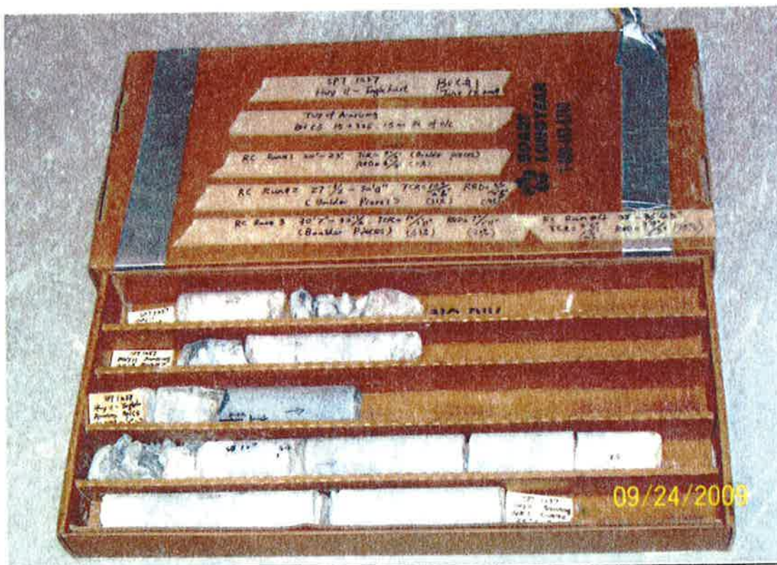
BH # C5 / Rock Core RC9 (6.1-7.0) m, RC12 (8.38-9.14) m, RC14 (9.32-9.91) m and Partial RC16 (10.06-11.08) m Depth
