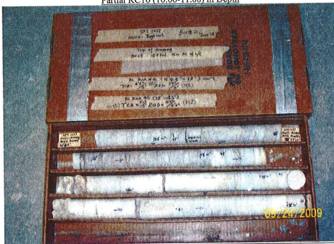
BH # C5 / Rock Core Partial RC16 (11.08-11.58) m, RC17 (11.58-13.11) m Depth
