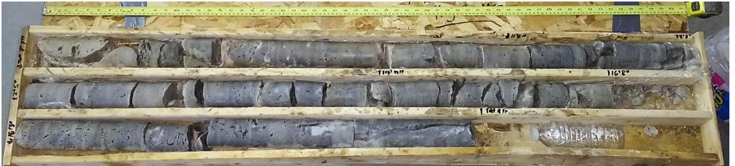
Rock Core Photos for Borehole 18-02: Run #1 (2.3 m – 3.4 m), Run #2 (3.4 m – 4.5 m) and Run #3 (4.5 m – 6.0 m)
