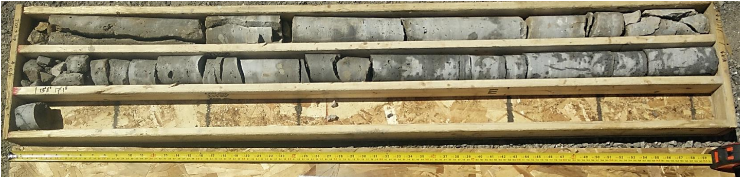
Rock Core Photos for Borehole 18-01: Run #1 (2.1 m – 3.6 m) and Run #2 (3.6 m – 5.2 m)
