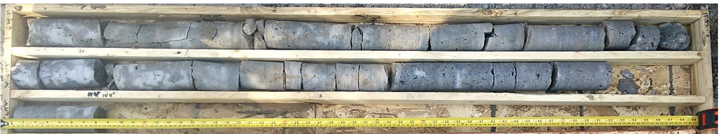
Rock Core Photos for Borehole 18-03: Run #1 (2.1 m – 3.6 m) and Run #2 (3.6 m – 5.1 m)
