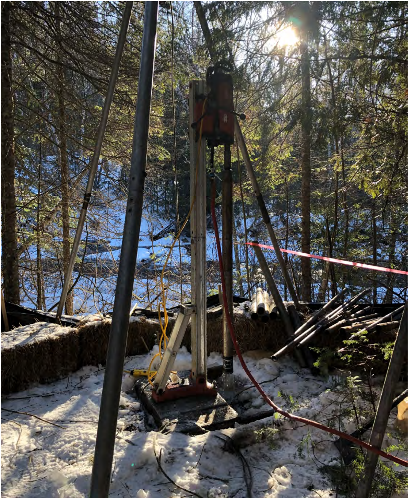
Photograph #18 – Hilti drilling and tripod setup at Borehole HEW-02 (January 2023)
