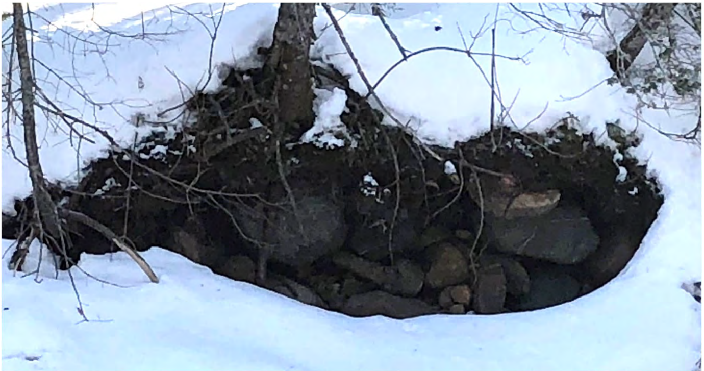
Photograph #8 – Exposed valley slope on east side of Hewitson Creek showing frequent boulders within the native overburden (January 2023)
