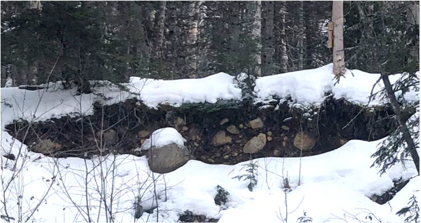
Photograph #7 – Exposed valley slope on east side of Hewitson Creek showing coarse gravel, cobbles, and boulder within the native overburden (January 2023)
