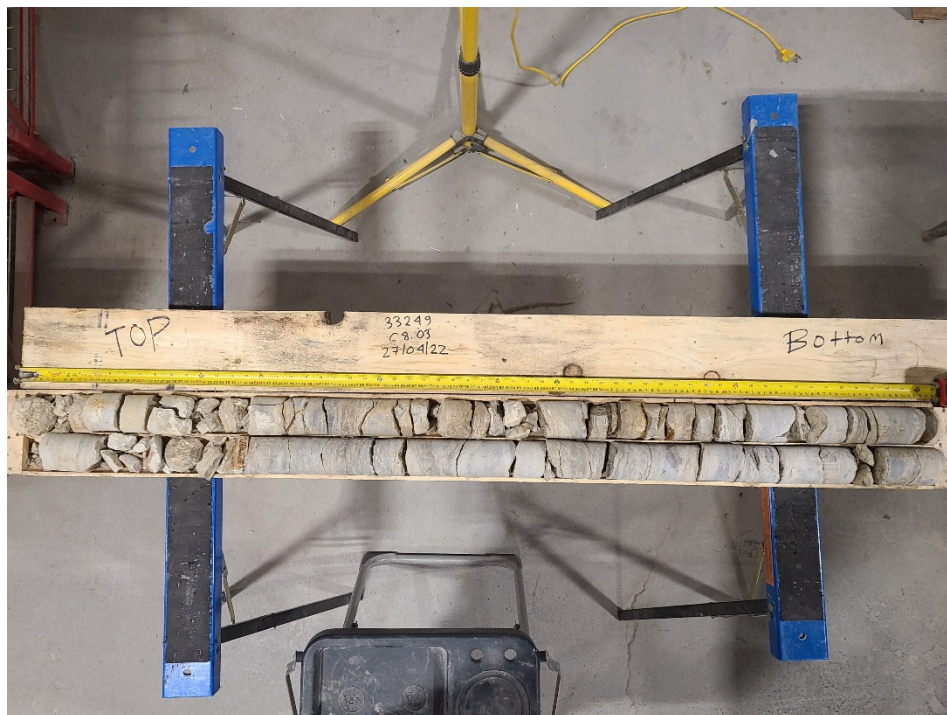
Photograph #6 – Bedrock Core Samples for Borehole C8-03
