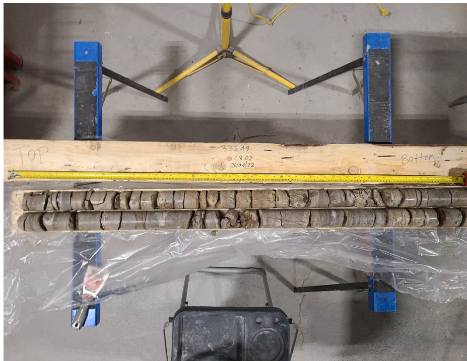
Photograph #5 – Bedrock Core Samples for Borehole C8-02
