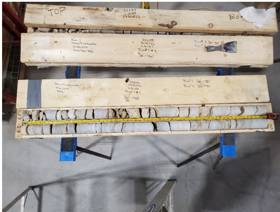
Photograph #3 – Bedrock Core Samples for Borehole C8-01
