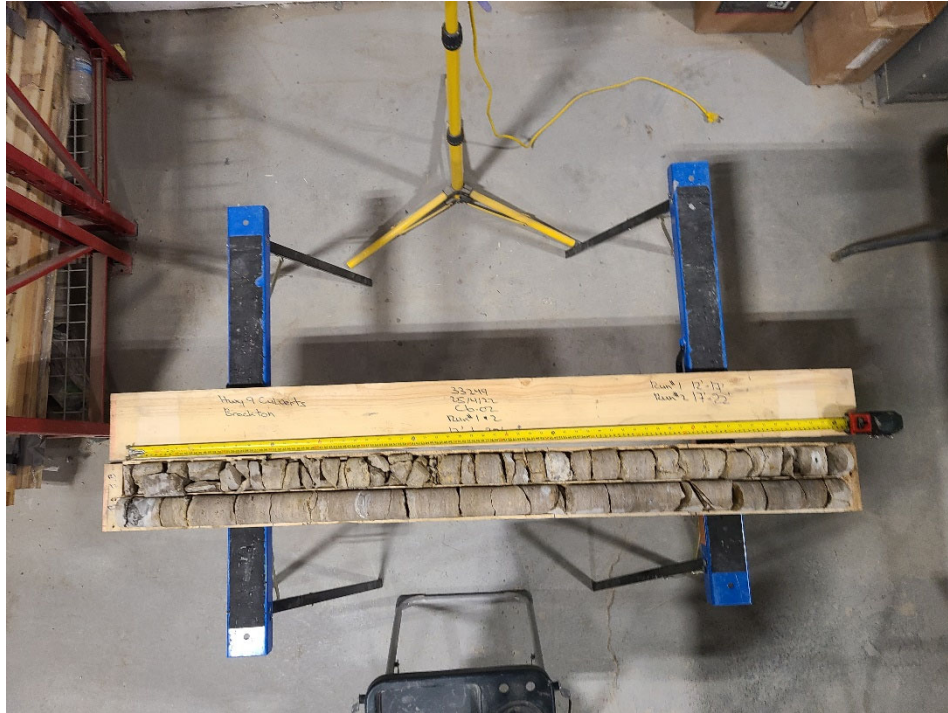
Photograph #5 – Bedrock Core Samples for Borehole C6-02
