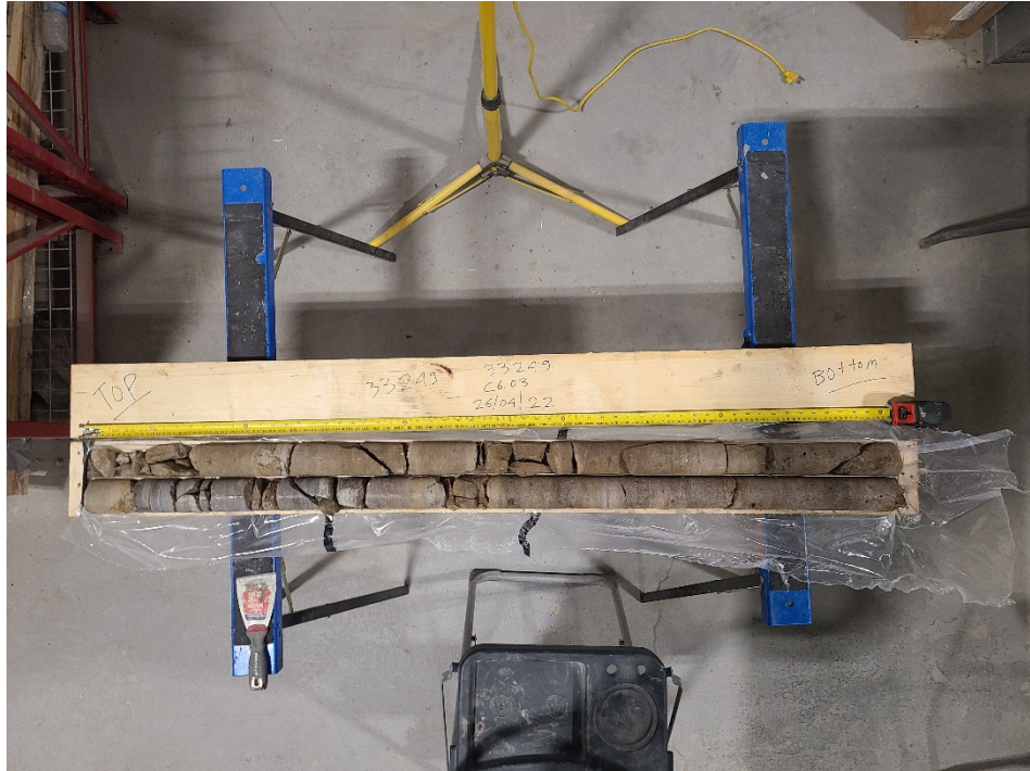
Photograph #6 – Bedrock Core Samples for Borehole C6-03
