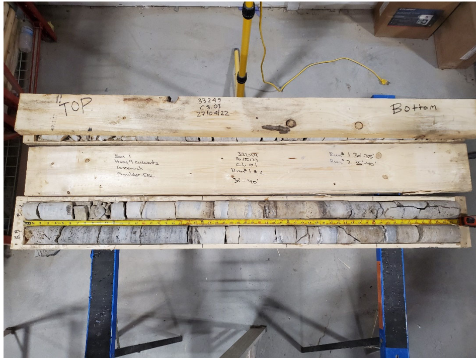
Photograph #3 – Bedrock Core Samples for Borehole C6-01
