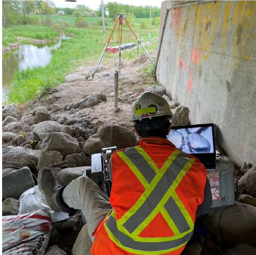
Photo 6: Looking South – Borehole Magnetometer Testing at Borehole 22-03
