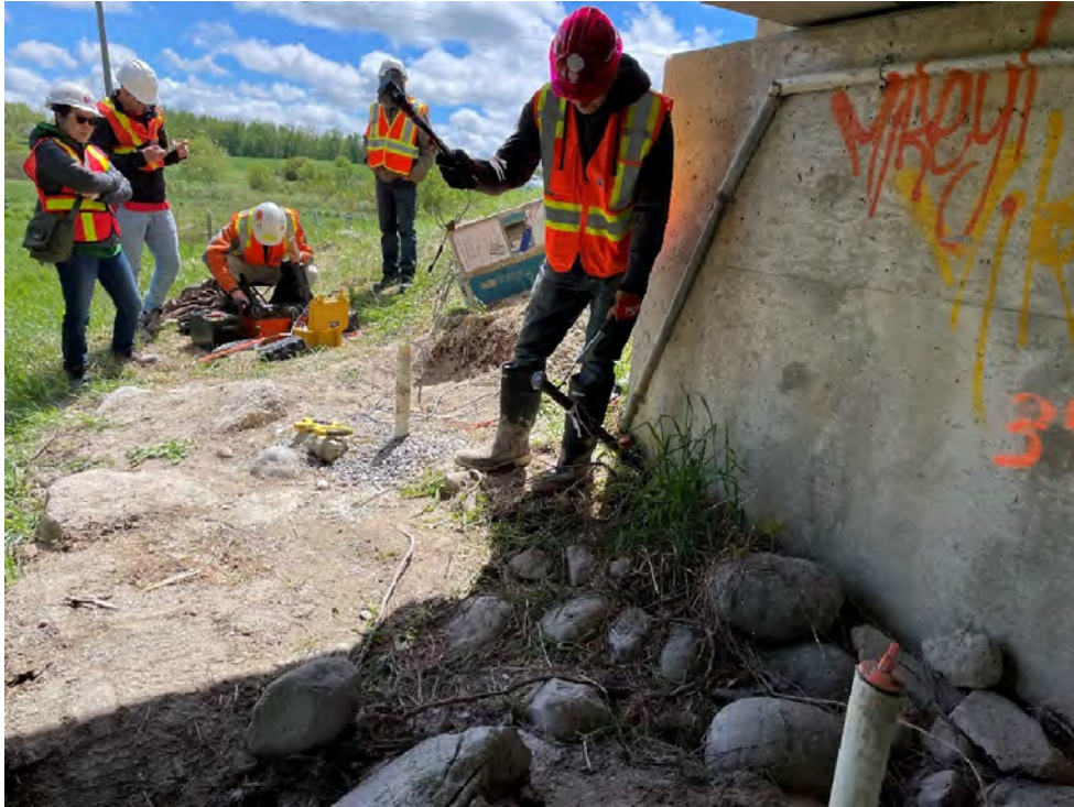
Photo 5: Looking south - Parallel Seismic Testing at Borehole 22-03 at west abutment
