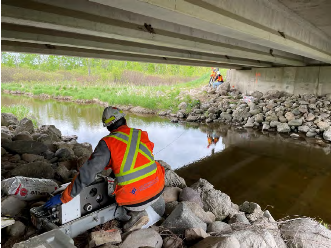
Photo 7: Looking northeast – Natural Gamma testing at Borehole 22-04
