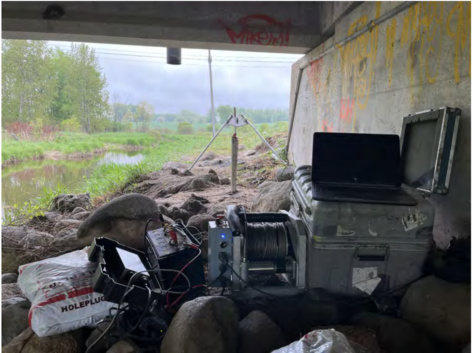
Photo 4: Magnetometer Survey in BH-05
