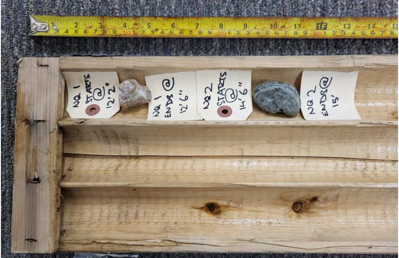
Photograph #8 – Core sample from AW1 and AW2 core of Borehole 21258-05. (October 2022)
