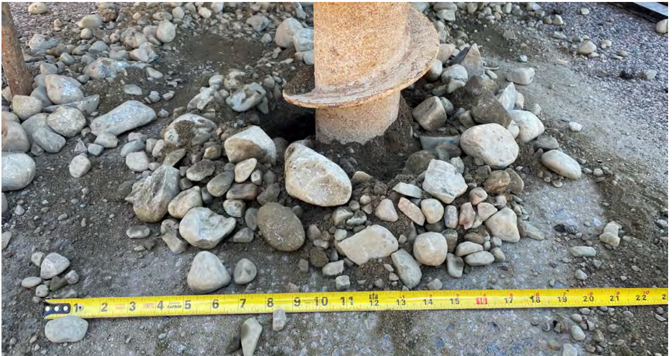
Photograph #8 – Soil cuttings from advancing borehole with augers in embankment fill at Borehole 18289-03. Note gravel and cobble-sized particles in soil cuttings.
