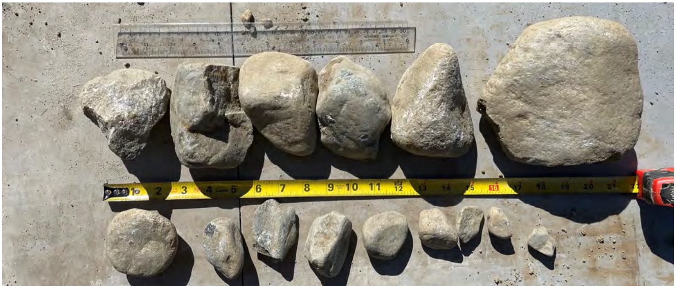
Photograph #9 – Selection of gravel and cobble sized particles recovered from embankment fill soil cuttings from advancing borehole 18289-03 with augers. Largest cobble dimension in above photograph is approximately 175 mm.
