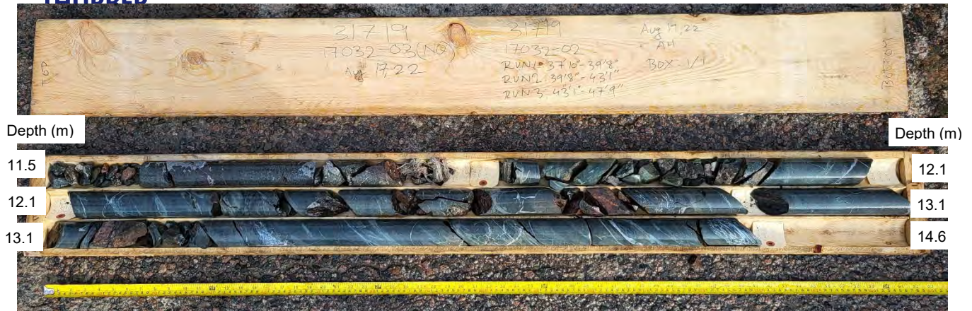
Photograph #5 – Rock Coring Runs 1, 2, and 3 of Borehole 17032-02
