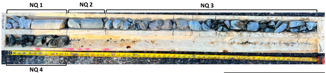
Borehole 19640-01 - Cored Gravels, and Cobbles
