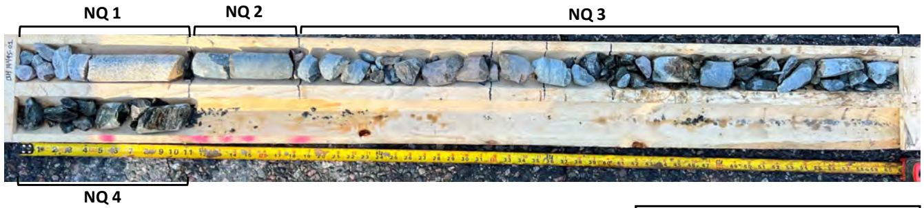
Borehole 19640-01 - Cored Gravels, and Cobbles
