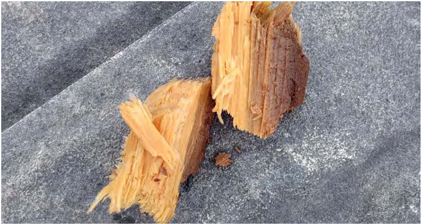
Photograph #6 – Wood fragments recovered in Borehole 10119-02 (December 2022)
