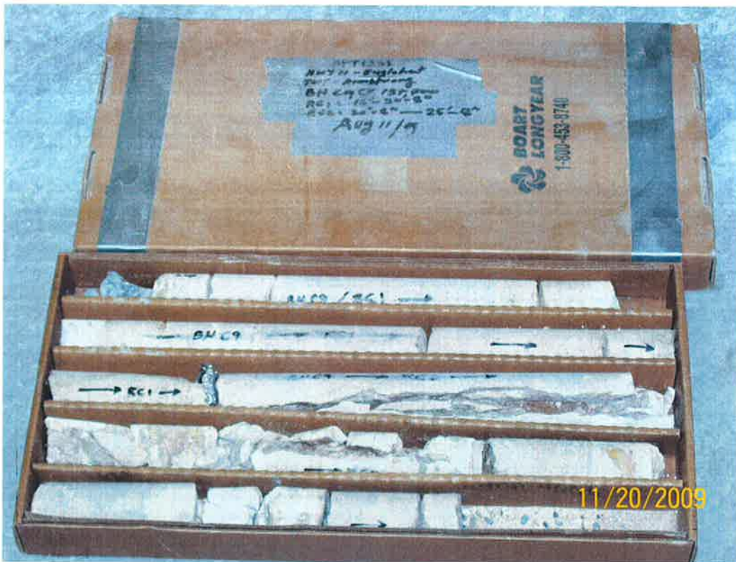
Figure E1 – Rock Core Sample (RC9) from Borehole C9 at Passing Lane 2
