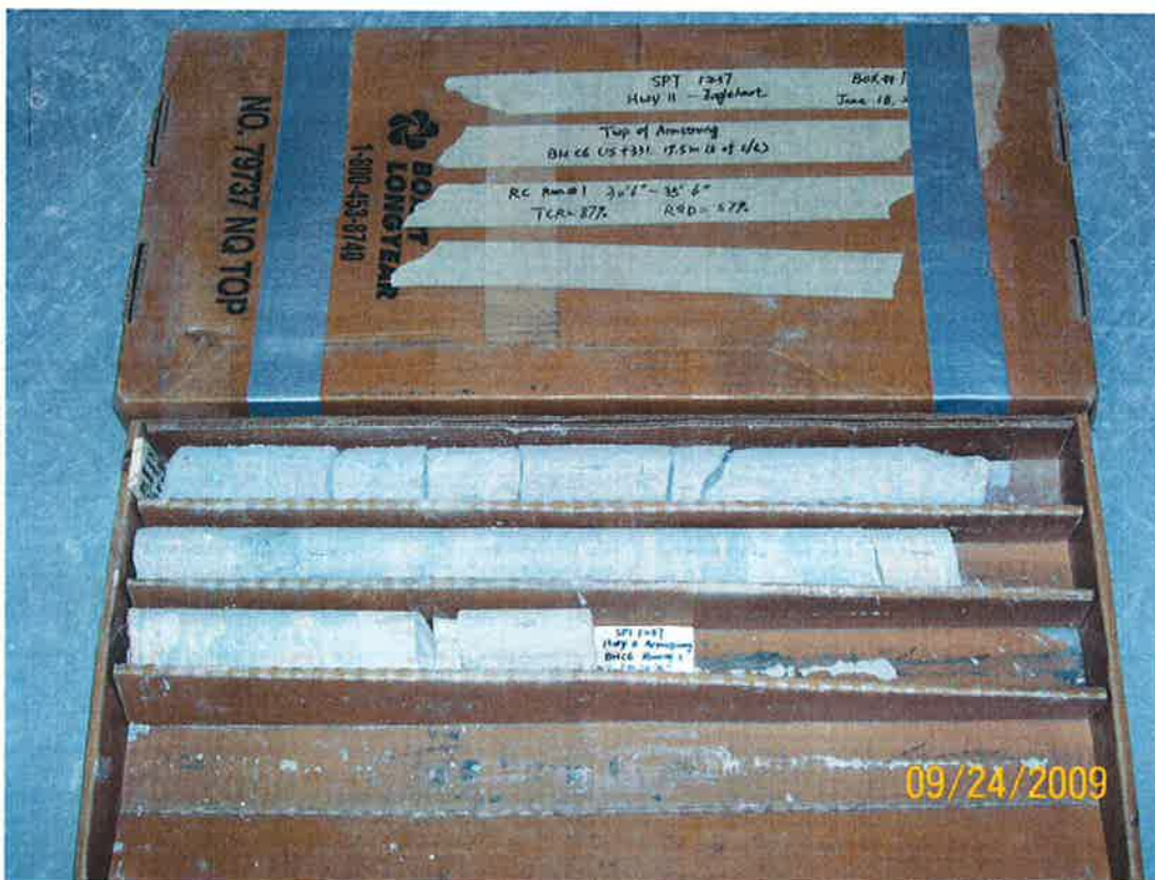
Figure E2 – Rock Core Sample (RC13) from Borehole C6 at Passing Lane 3
