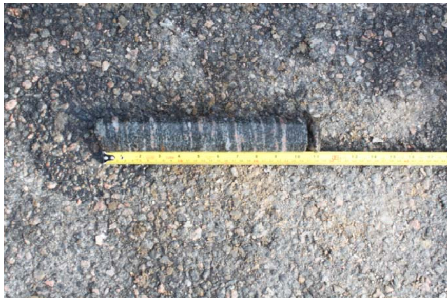
Photo 8. The core of gneiss boulder recovered from BH-13A
