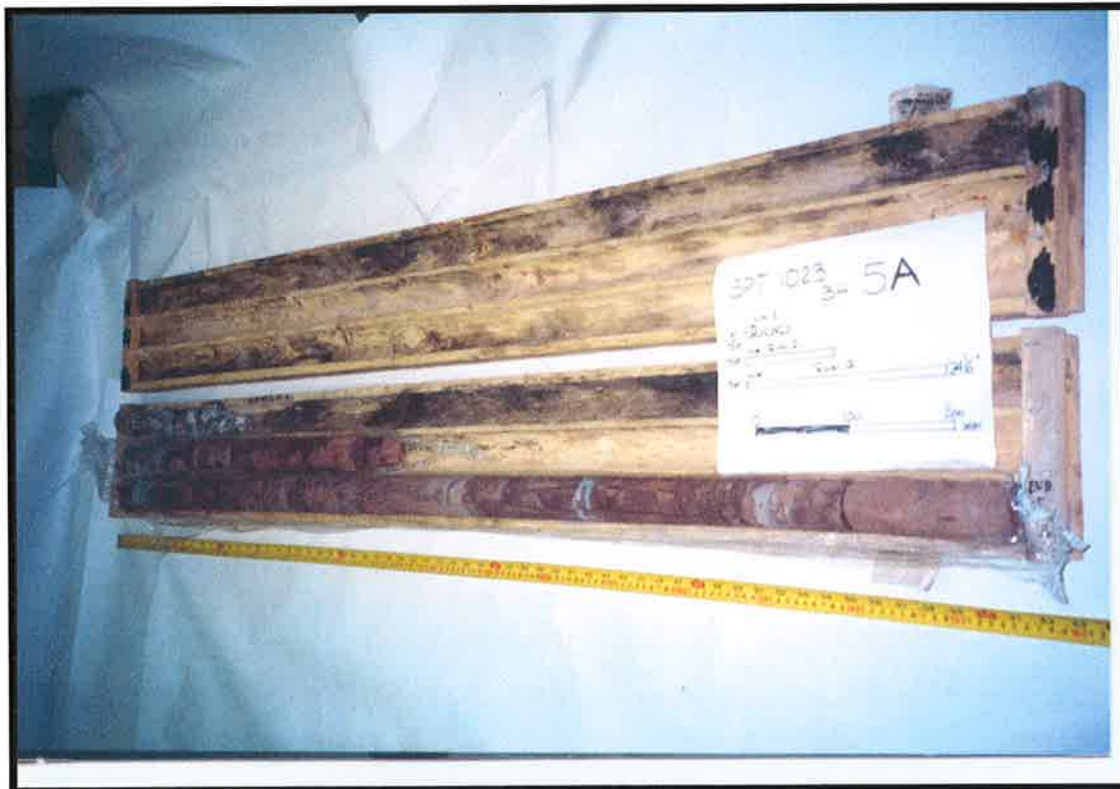
PHOTOGRAPHS OF CORE IN BOREHOLES 4A AND 5A (BH4A: ELEVATION 183.1 TO 181.8 M) (BH5A: ELEVATION 183.3 TO 181.2 M)
