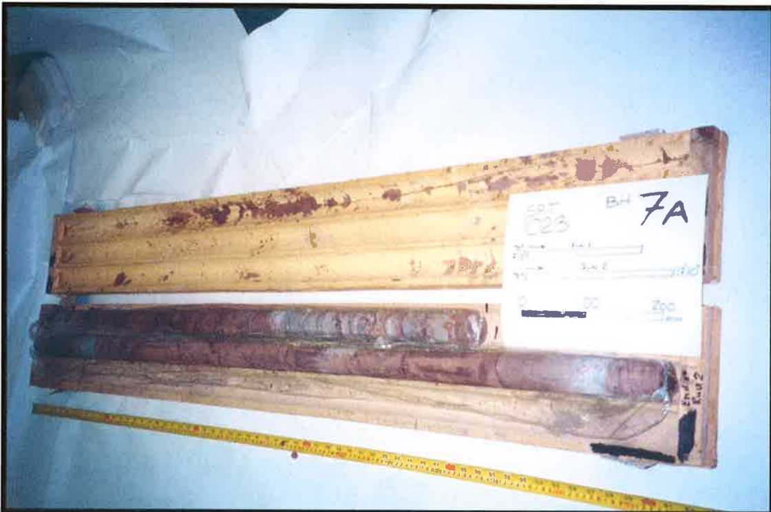
PHOTOGRAPHS OF CORE IN BOREHOLES 6 AND 7A (BH6: ELEVATION 186.4 TO 183.9 M) (BH7A: ELEVATION 186.0 TO 183.0 M)
