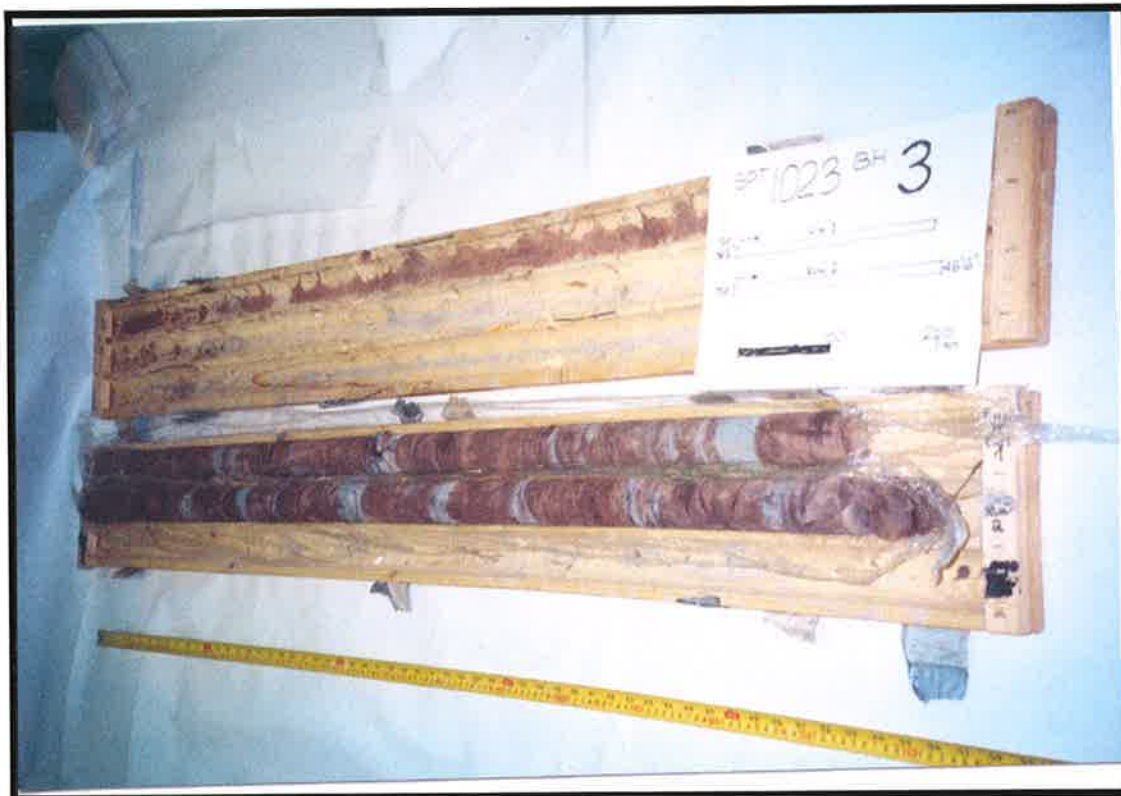
PHOTOGRAPHS OF CORE IN BOREHOLES 2 AND 3 (BH2: ELEVATION 182.4 TO 179.5 M) (BH3: ELEVATION 182.5 TO 179.4 M)
