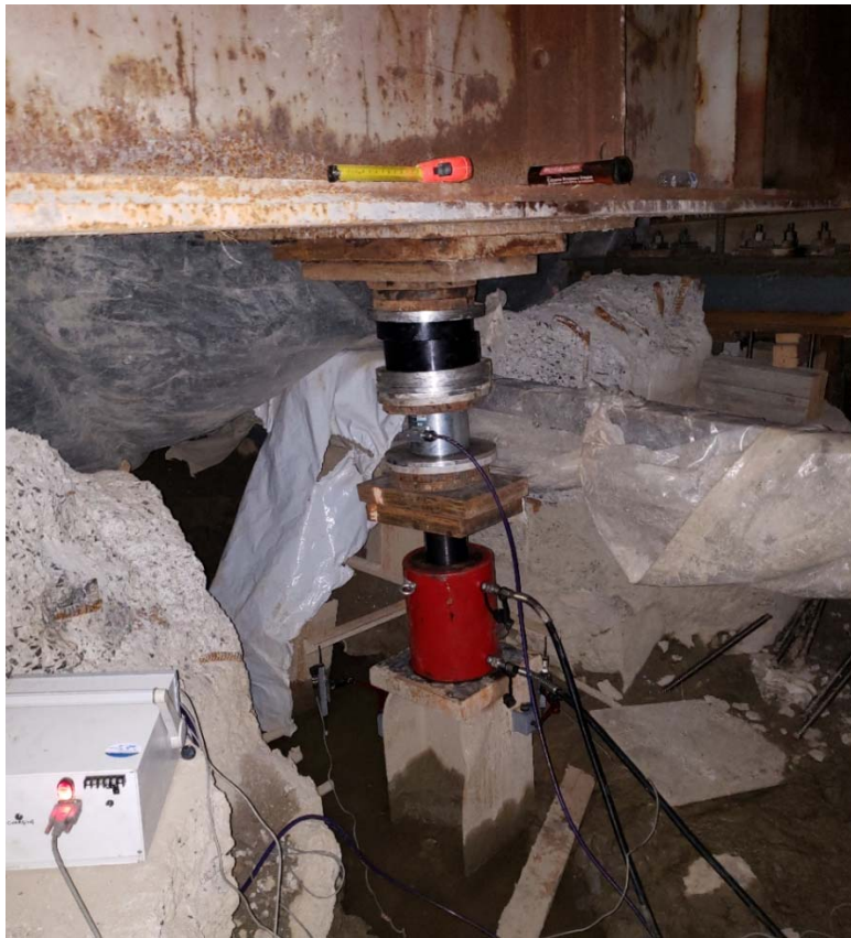
Figure 1. Pile, instrumentation, and reaction system
