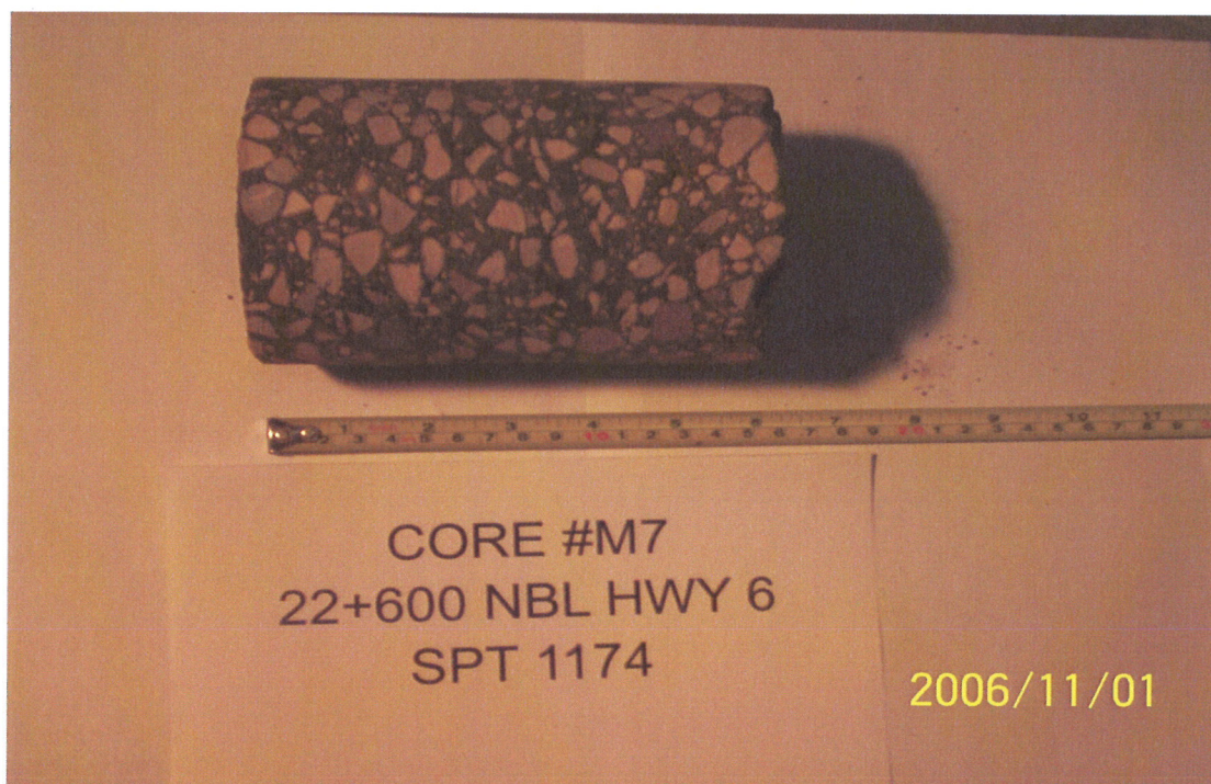
Photograph 4- Core No.M7 at 22+600, NBL, Highway 6
