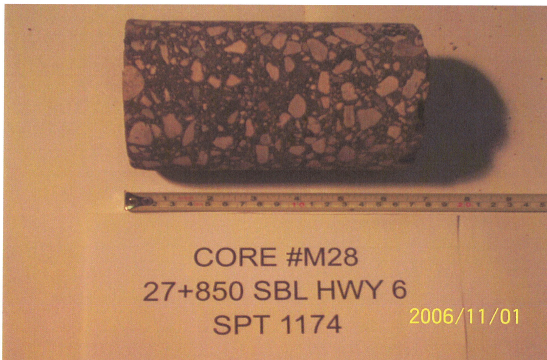
Photograph 10- Core No.M28 at 27+850, SBL, Highway 6
