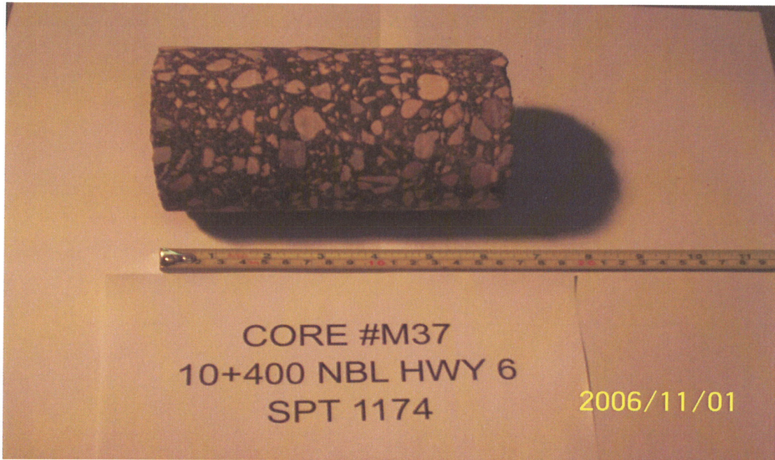
Photograph 1- Core No.M37 at 10+400, NBL, Highway 6
