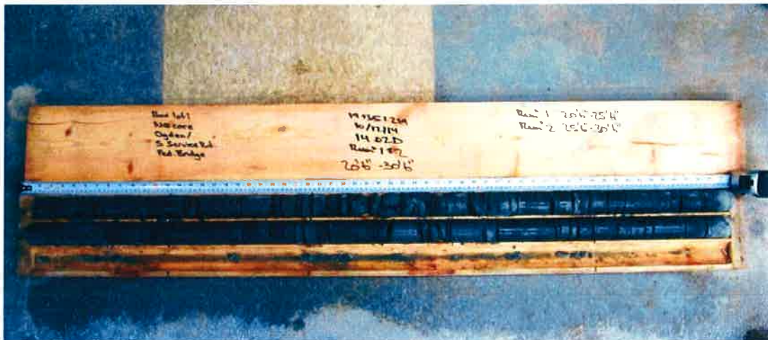
Photograph 2 – Rock Core from Drillhole 14-02
