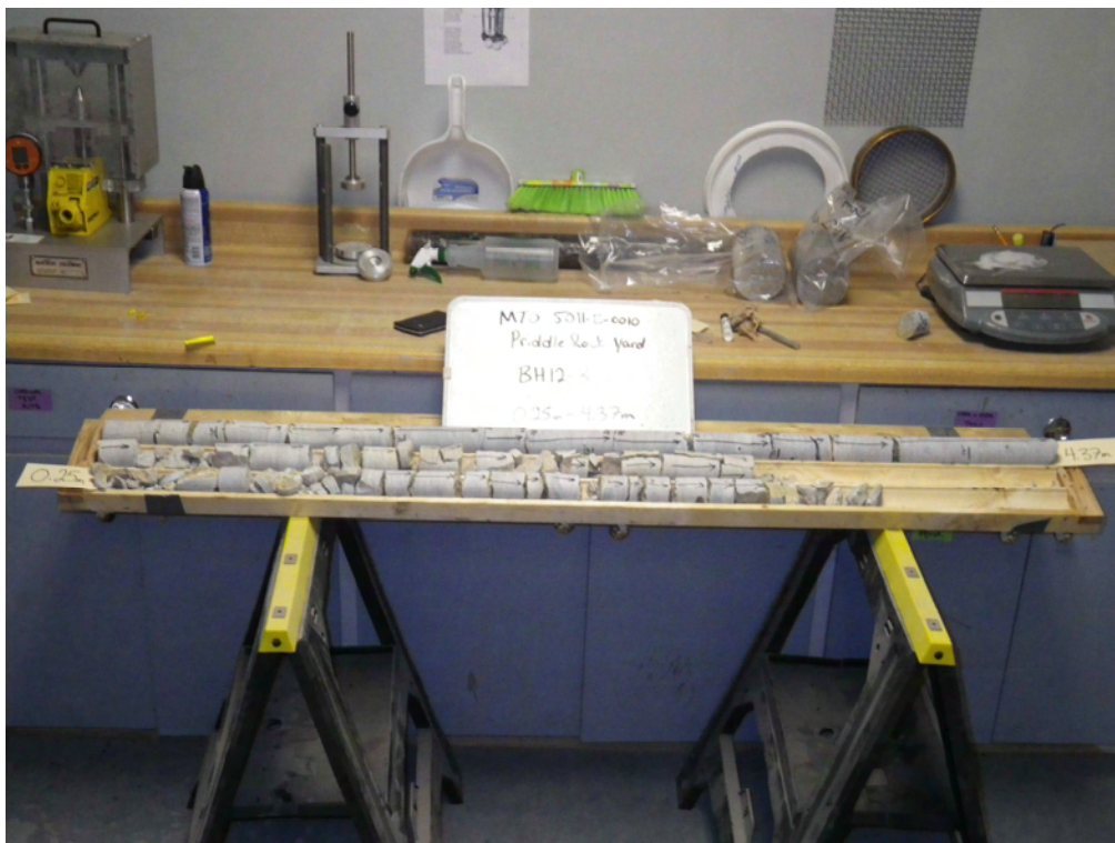
Photograph 2: BH12-3 Rock Core (0.25 m to 4.37 m).
