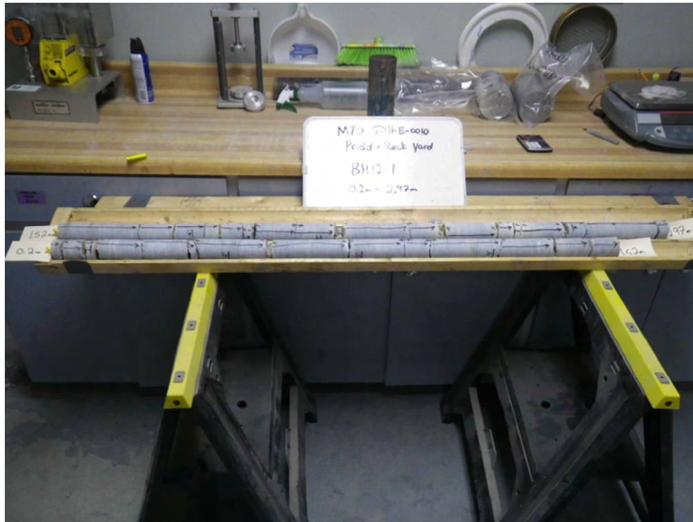
Photograph 1: BH12-1 Rock Core (0.2 m to 2.97 m).
