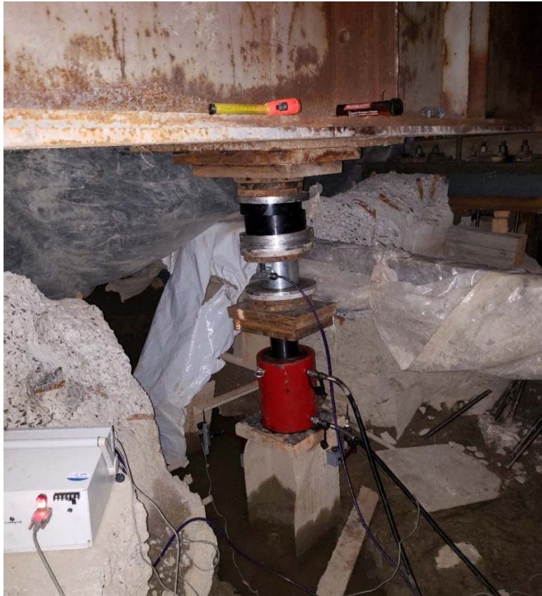
Figure 1. Pile, instrumentation, and reaction system
