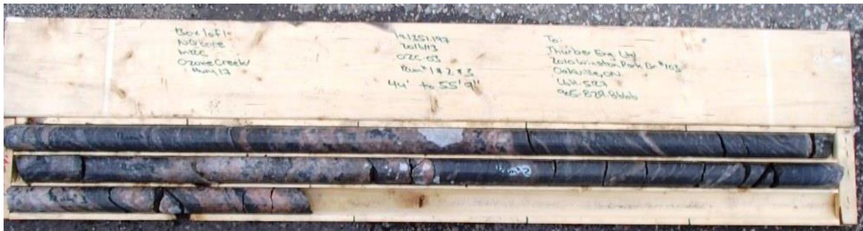
Photograph 2 – Rock core recovered from Borehole OZC-03
