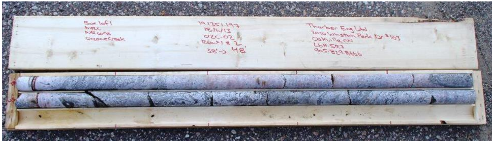
Photograph 1 – Rock core recovered from Borehole OZC-02
