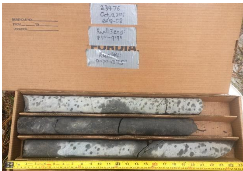
Photo B19: Borehole 18-08 core photo. Run 3 end to Run 4.
