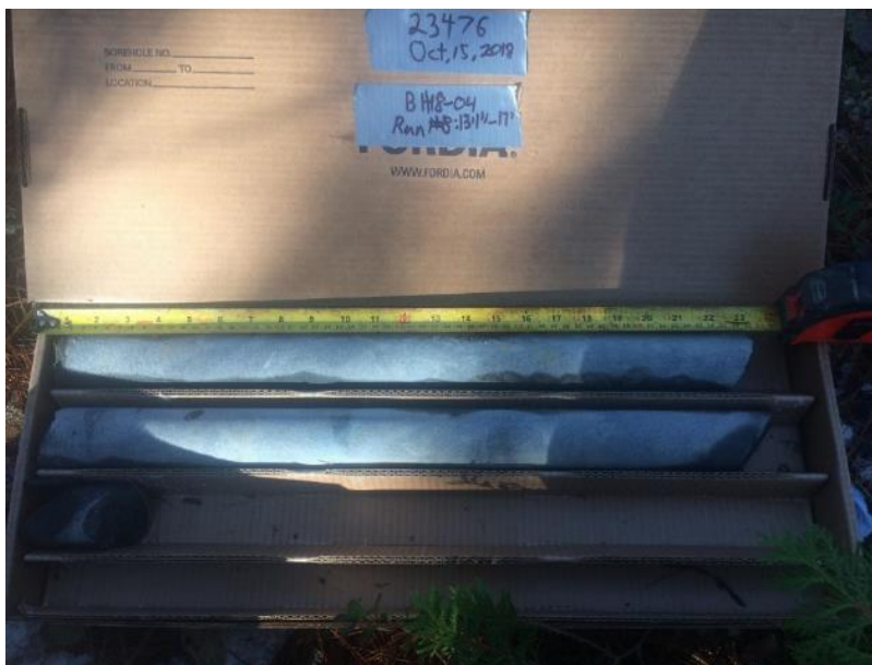
Photo B9: Borehole 18-04 core photo. Run 6 end to Run 7.
