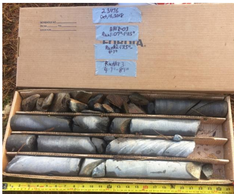
Photo B5: Borehole 18-02 core photo. Run 4 end to Run 5.
