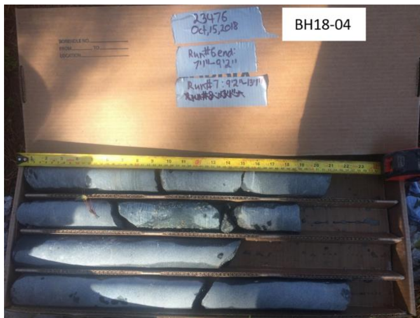
Photo B9: Borehole 18-04 core photo. Run 6 end to Run 7.
