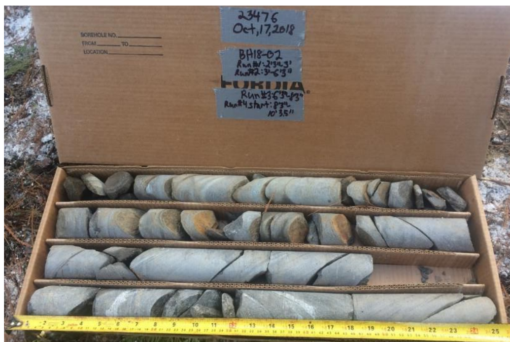
Photo B3: Borehole 18-01 core photo. Run 6 end.
