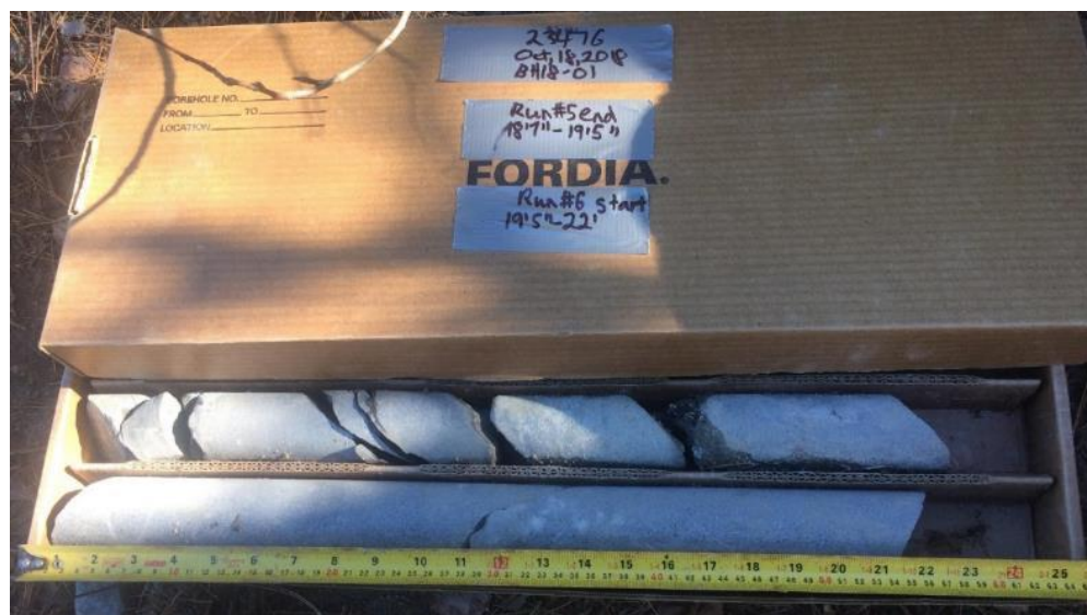
Photo B1: Borehole 18-01 core photo. Run 1 to Run 5 start.
