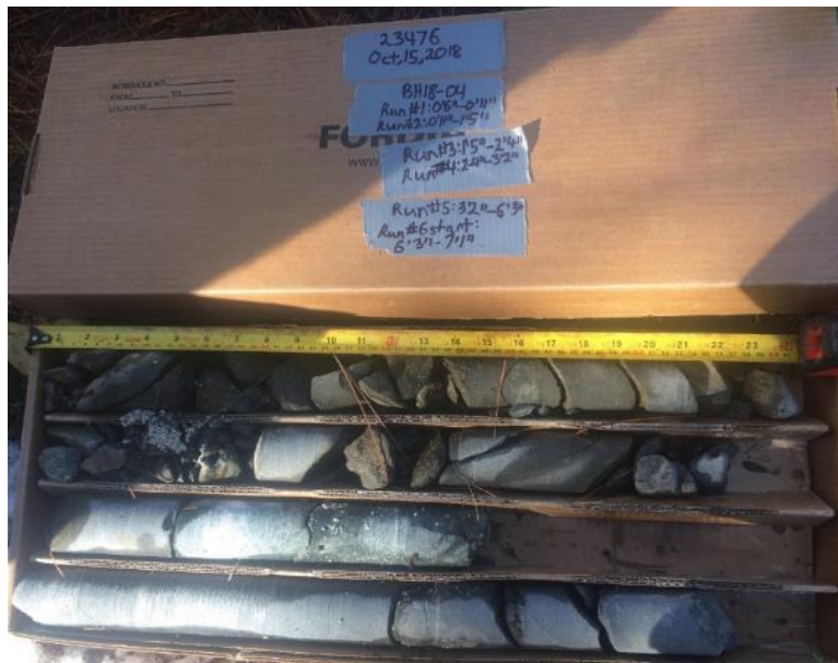
Photo B7: Borehole 18-03 core photo. Run 4
