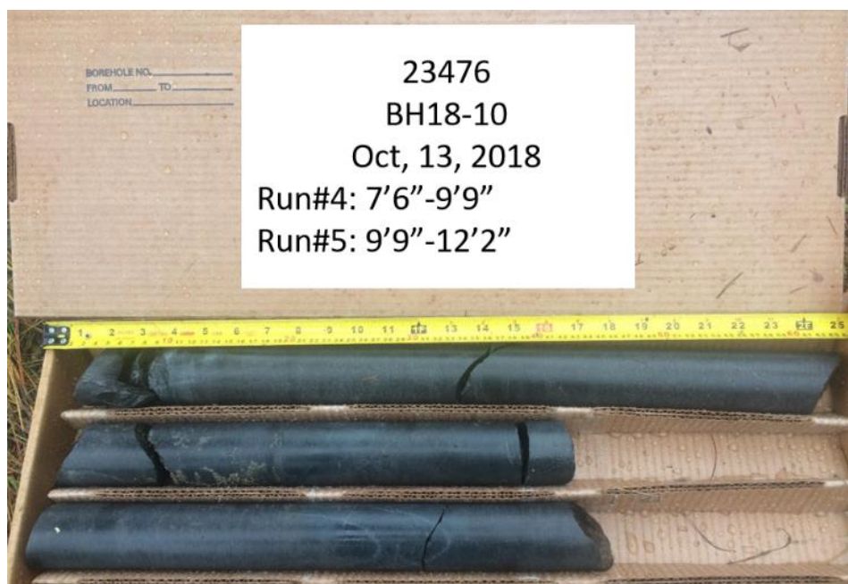
Photo B23: Borehole 18-10 core photo. Run 4 to Run 5
