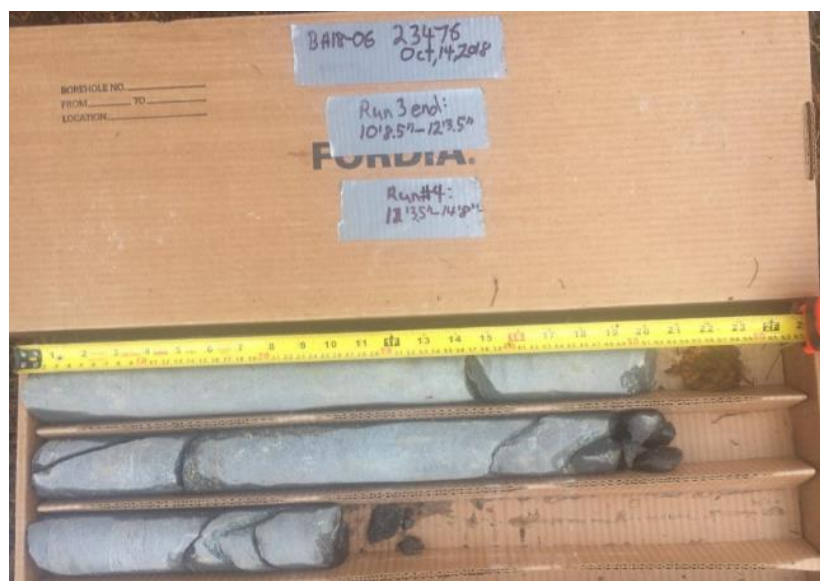
Photo B15: Borehole 18-06 core photo. Run 3 end to Run 4.
