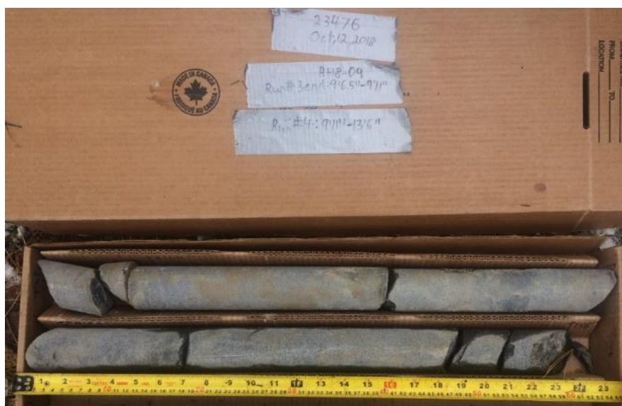
Photo B21: Borehole 18-09 core photo. Run 3 end to Run 4.
