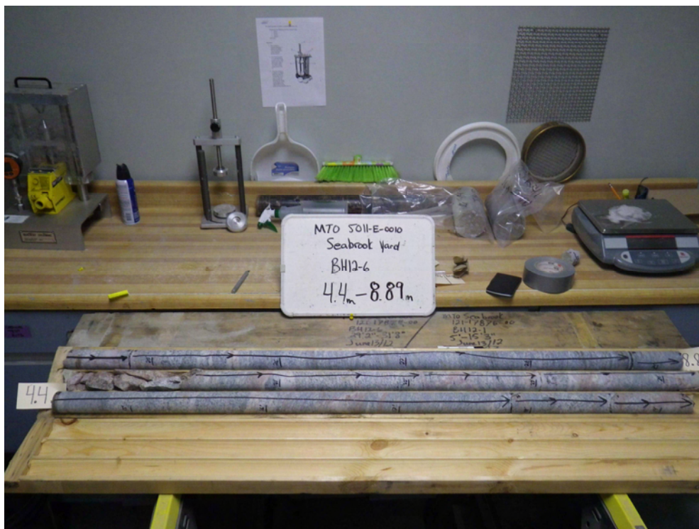
Photograph 9: BH12-6 Rock Core (4.4 m to 8.89 m).
