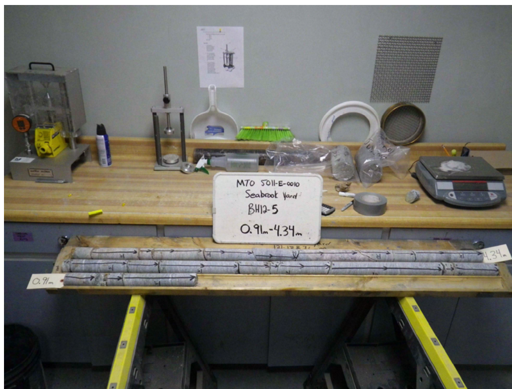
Photograph 6: BH12-5 Rock Core (0.91 m to 4.34 m).
