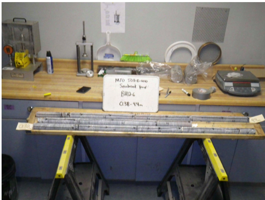
Photograph 7: BH12-6 Rock Core (0.38 m to 4.4 m).
