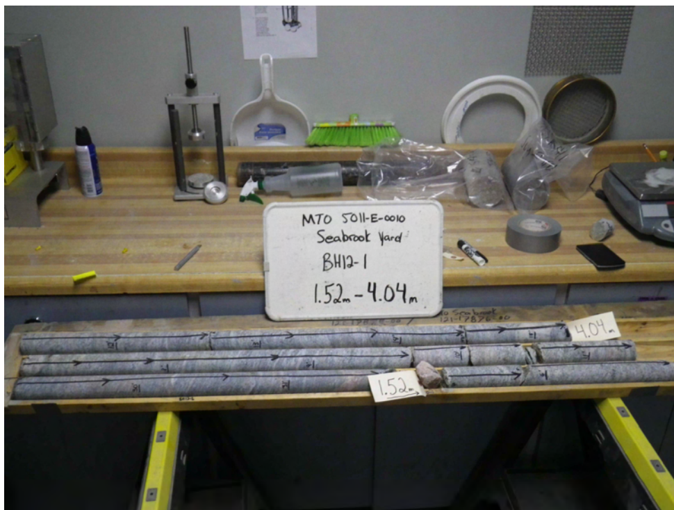
Photograph 1: BH12-1 Rock Core (1.52 m to 4.04 m).
