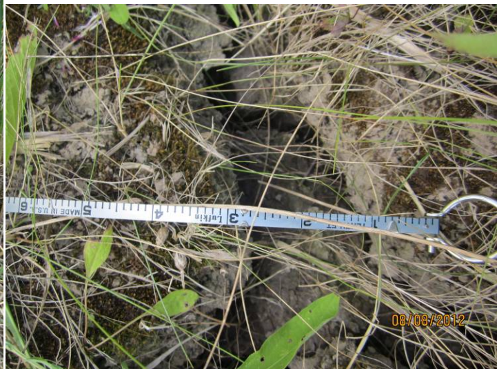
Figure 7: Width of the tension crack at the slope toe
