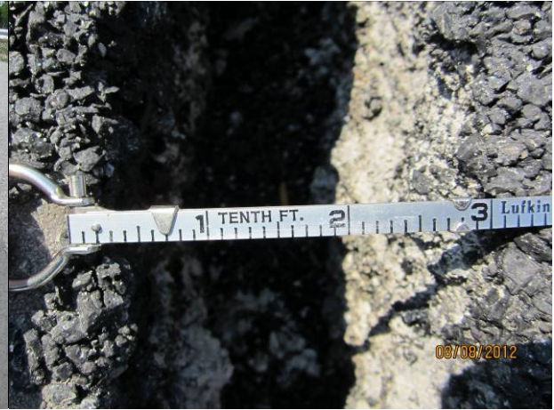
Figure 3: Width of the tension crack
