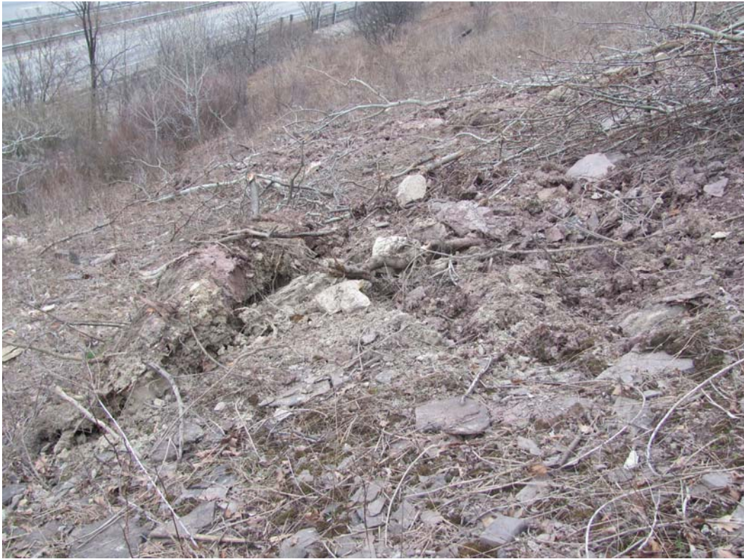
Image 19. Strike mark on slope below main failure, indicating that the long axis of the block was parallel to the slope and that the slope materials were saturated at the time of failure. (Image date – 29 March 2012)
