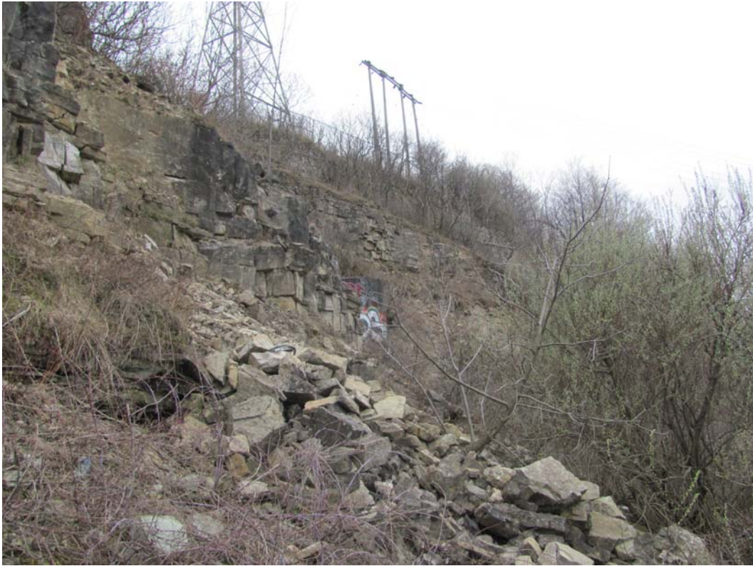
Image 17. Fresh looking talus pile below failed rock just to east of power lines. (Image date – 29 March 2012)
