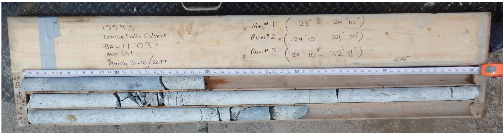
Photo 12: Borehole 17-03 Bedrock Core Sample
