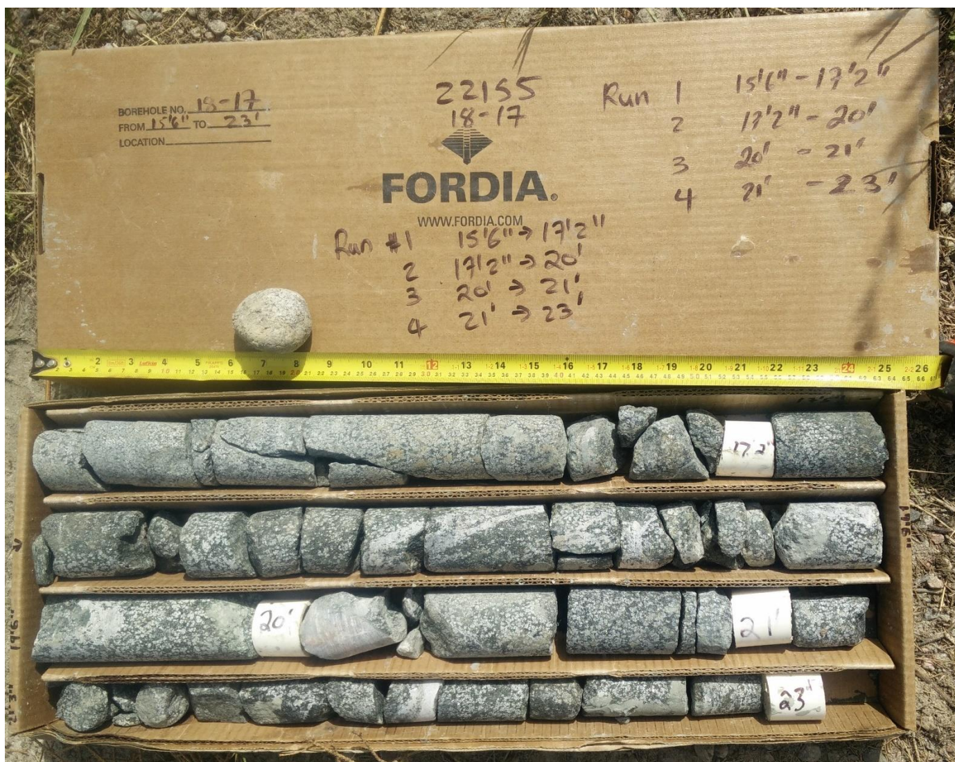
Photo 3: Borehole 18-17 Bedrock Core Sample
