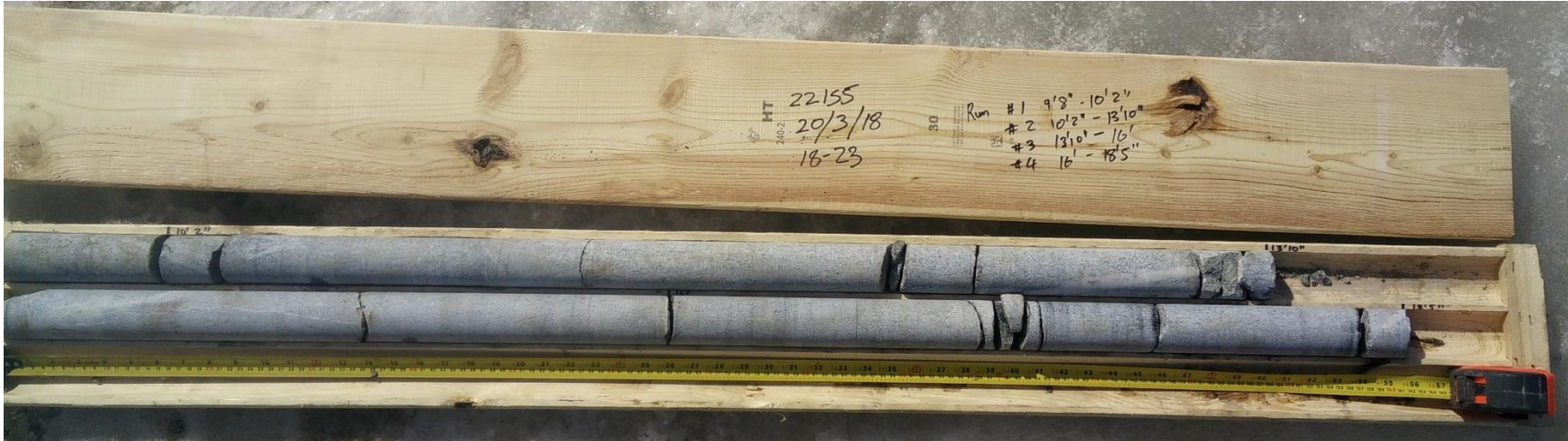
Photo 9: Borehole 18-23 Bedrock Core Sample
