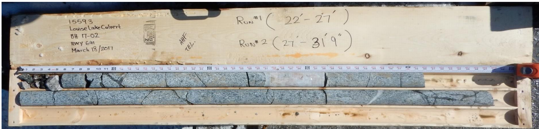
Photo 11: Borehole 17-02 Bedrock Core Sample
