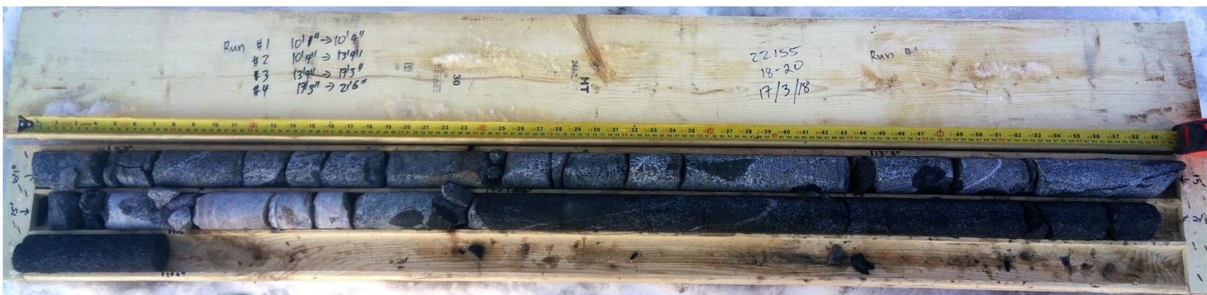
Photo 6: Borehole 18-20 Bedrock Core Sample
