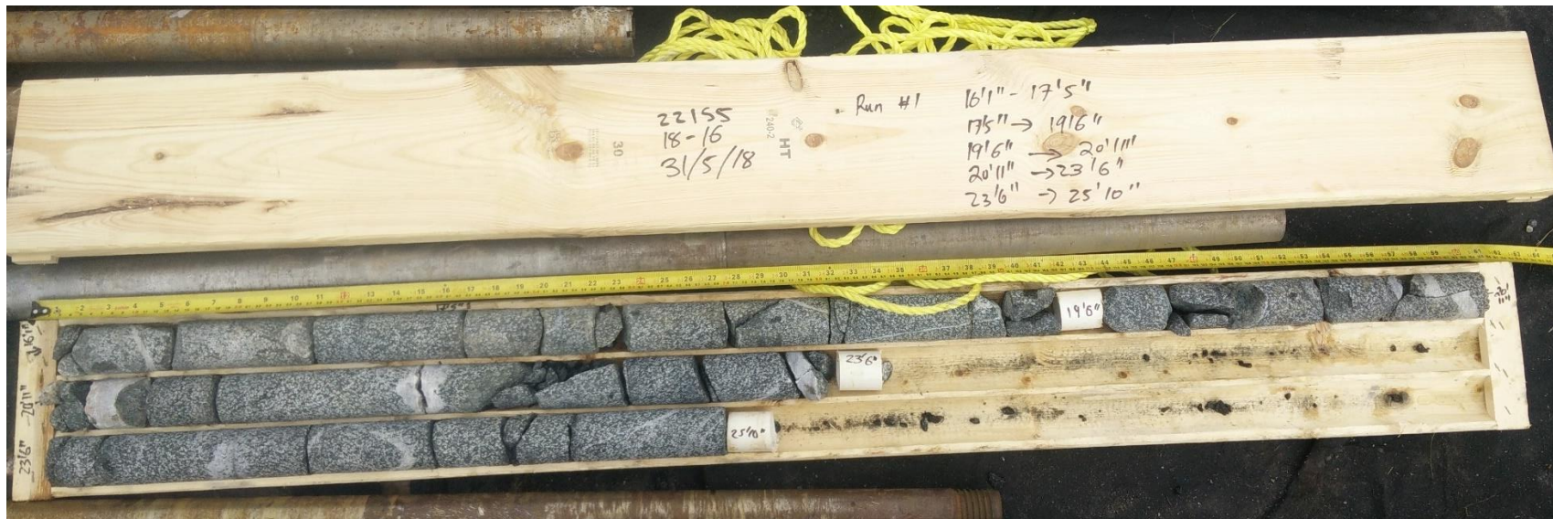
Photo 2: Borehole 18-16 Bedrock Core Sample
