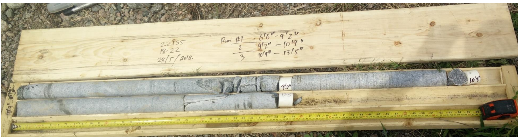
Photo 8: Borehole 18-22 Bedrock Core Sample
