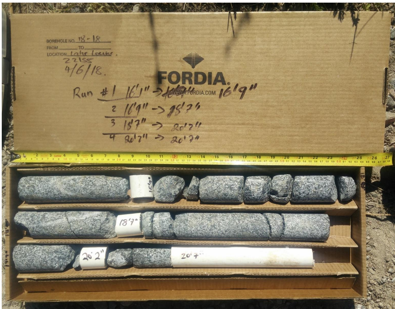
Photo 4: Borehole 18-18 Bedrock Core Sample
