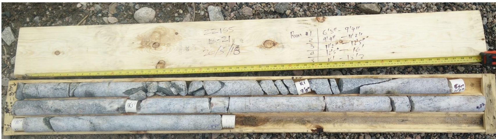
Photo 7: Borehole 18-21 Bedrock Core Sample
