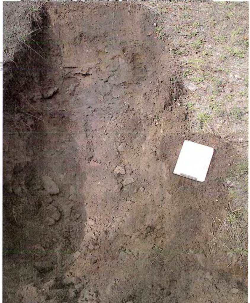
Photo: Test Pit 3 Embankment Fill
