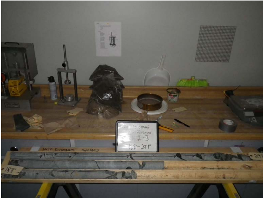
Photograph 3: BH12-3 Rock Core (5.55 m to 8.85 m).
