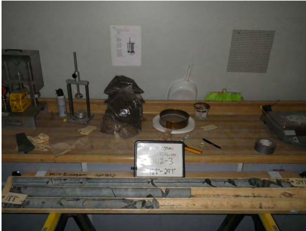
Photograph 3: BH12-3 Rock Core (5.55 m to 8.85 m).
