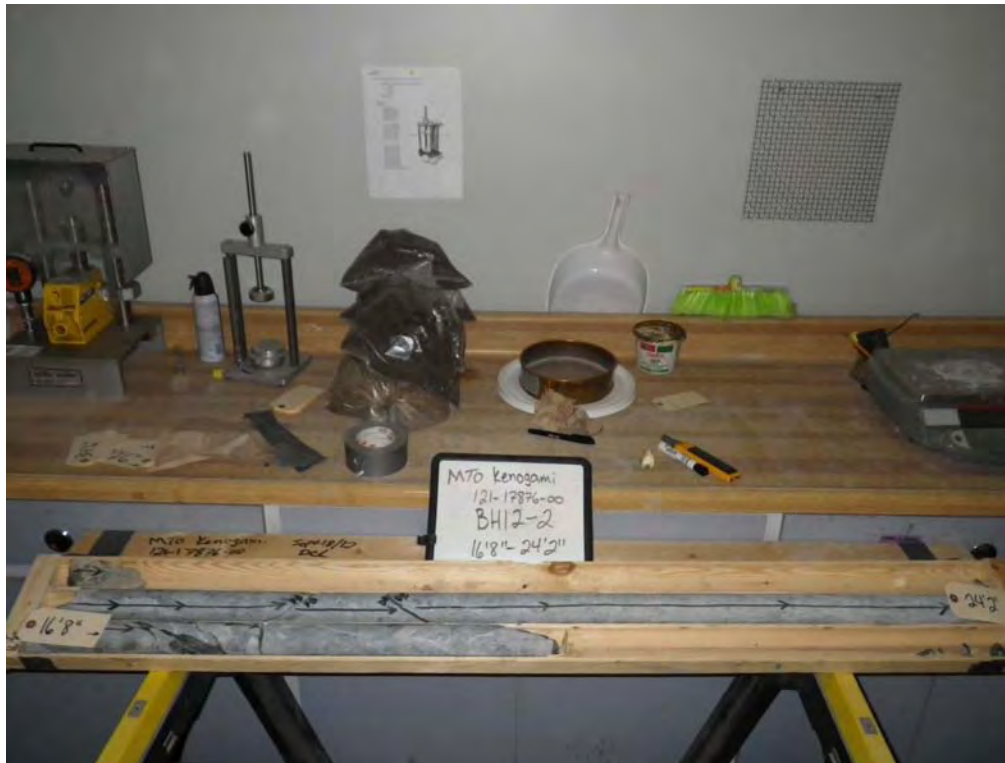
Photograph 1: BH12-2 Rock Core (4.94 m to 7.33 m).
