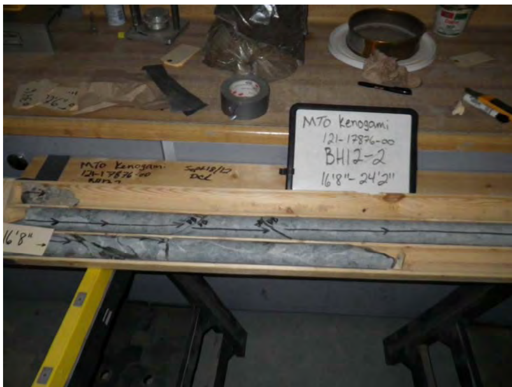
Photograph 2: BH12-2 Rock Core (4.94 m to 7.33 m).
