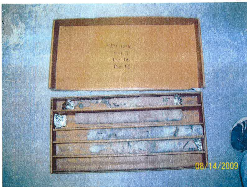
Photograph E3. Rock cores (RC15 and 16, BH B3)
