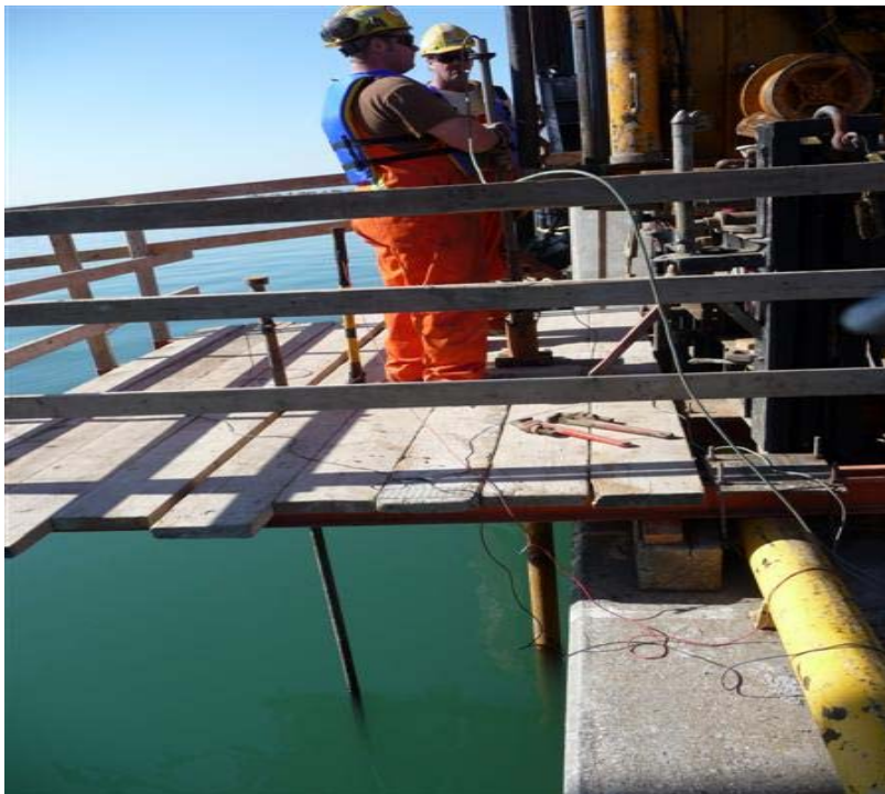
Fig.1. Picture of Cone Penetrometer Shear Wave Testing using the overwater platform. The platform was used for both CPT and PMT.
