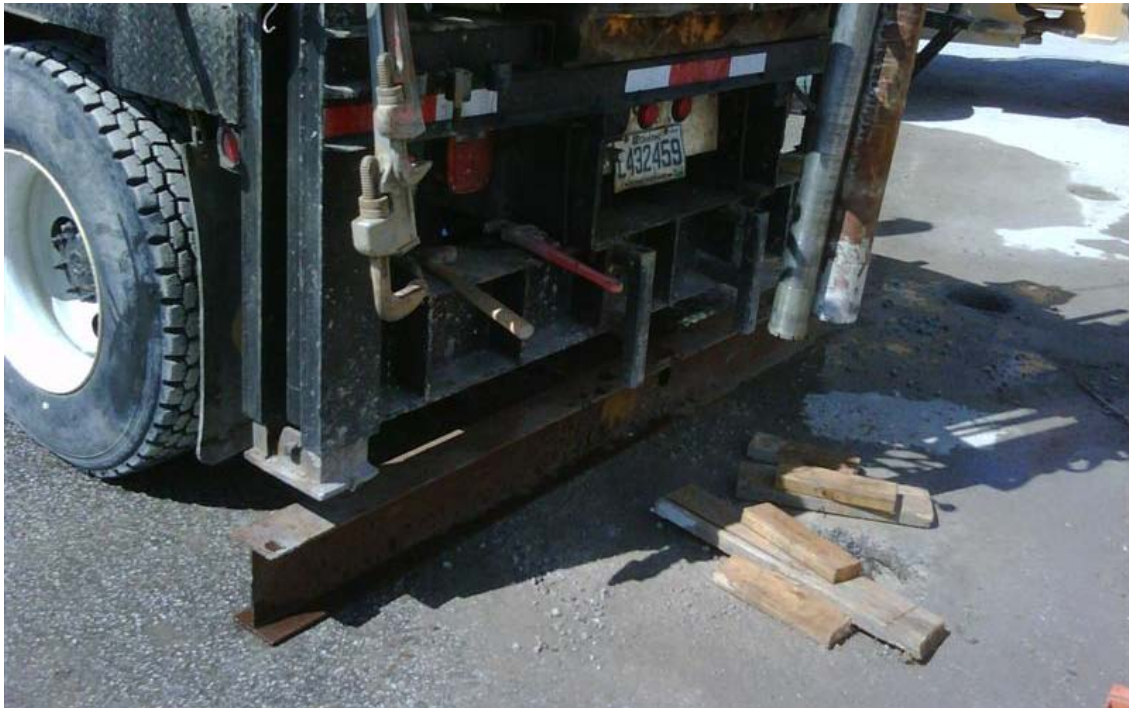
Figure 5 – Shear wave beam under drill rig outriggers prior to testing
