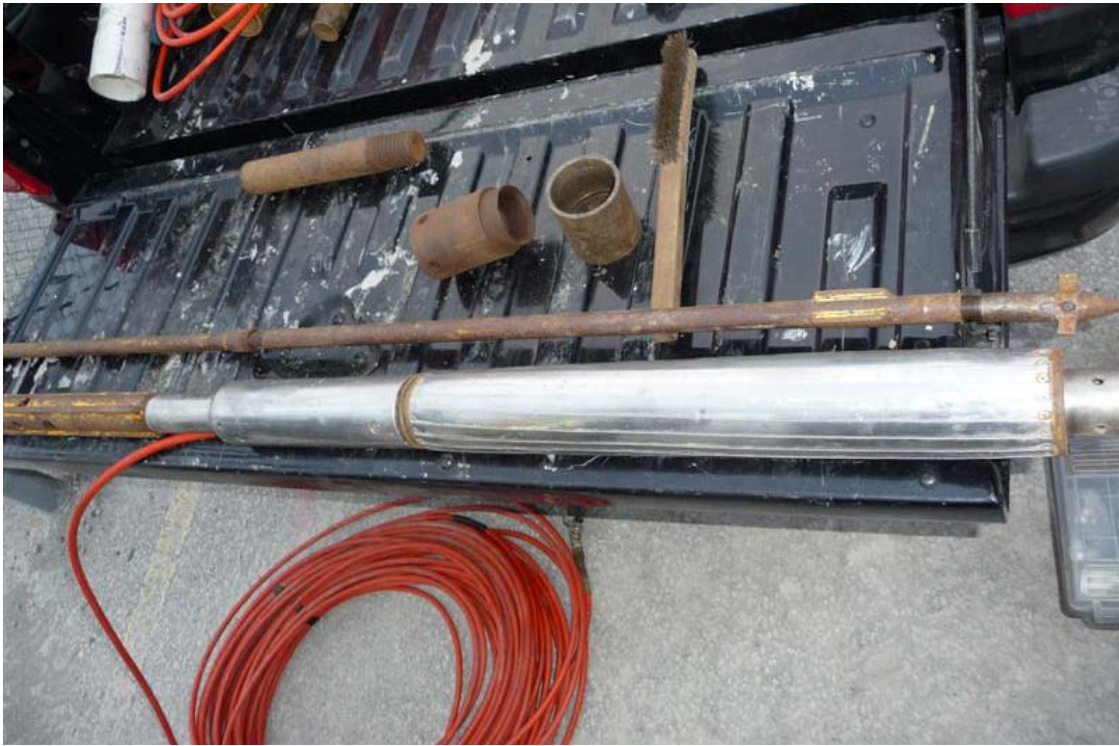
Figure 9 – Self-Bore Pressuremeter and jetting tool (unassembled)
