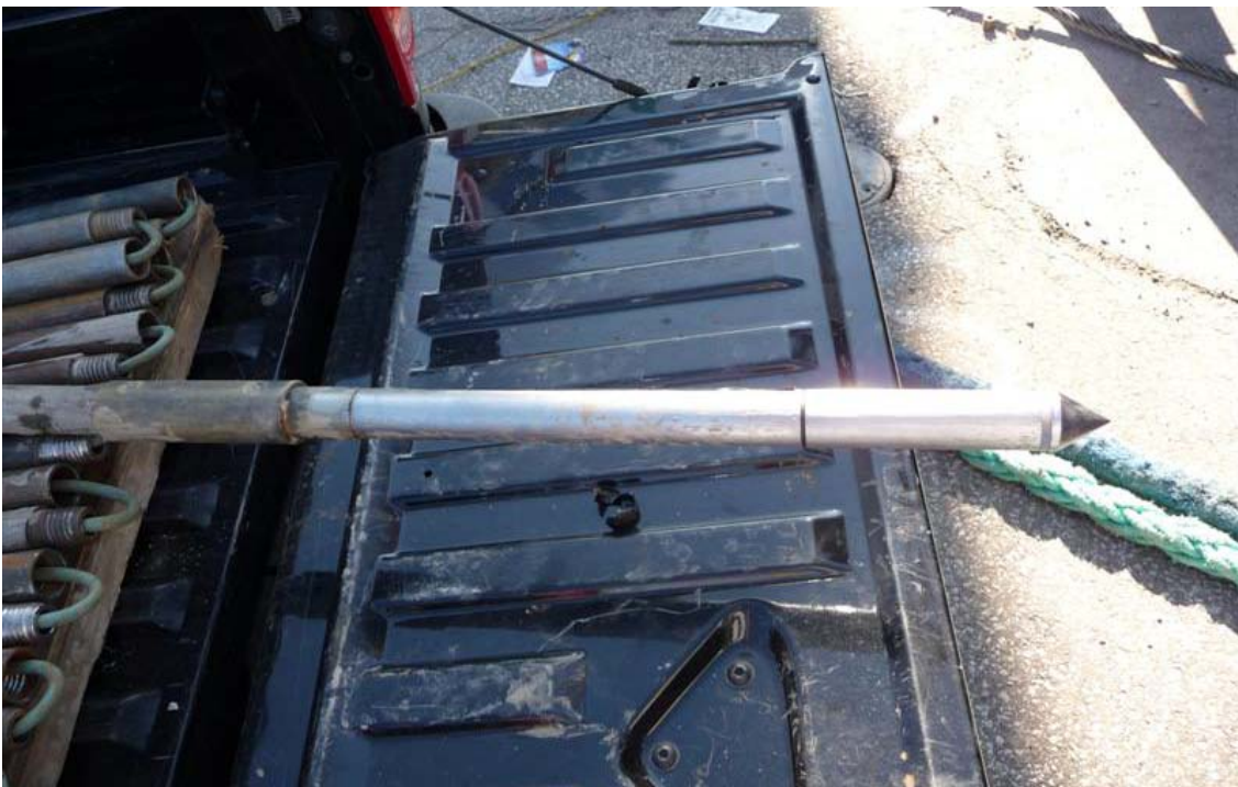
Figure 4 – CPT(u) prior to testing at (09-03N)
