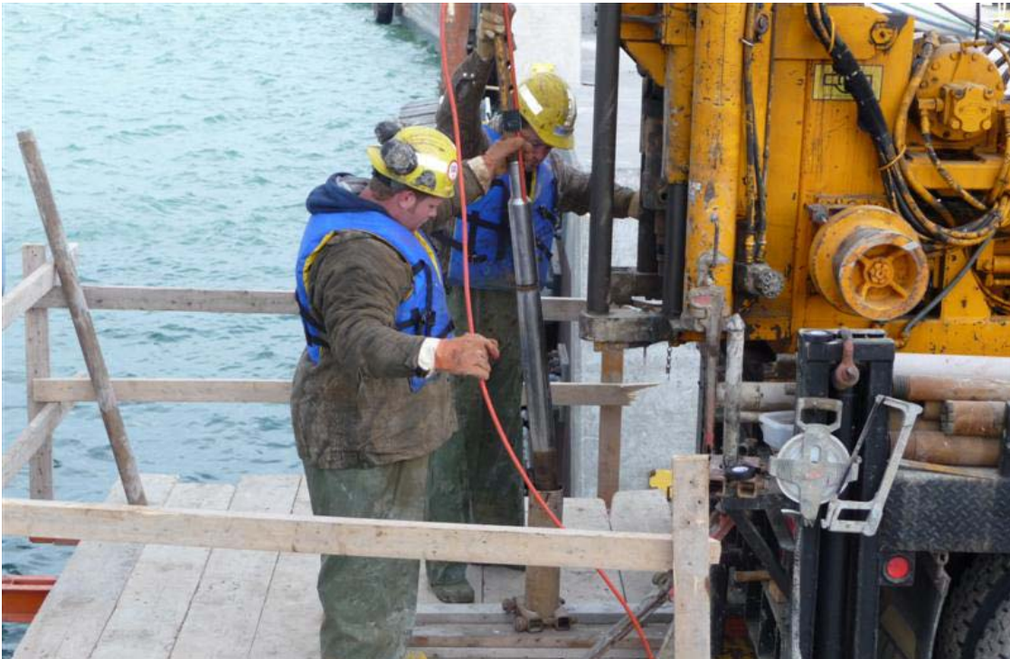
Figure 11 – Downhole insertion of the SBMP (09-02S)
