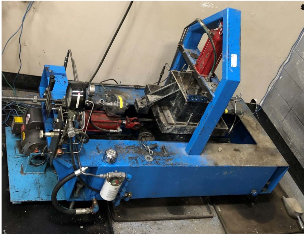
Figure 1: Golder's Large-Scale Direct Shear box in Calgary, AB.
