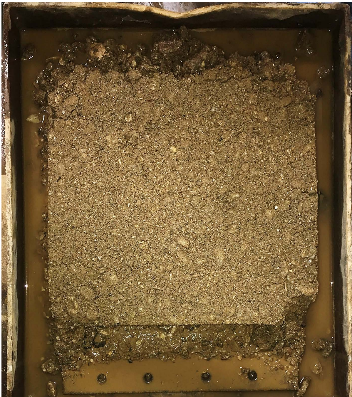
Post-Test Photo - 150 kPa
