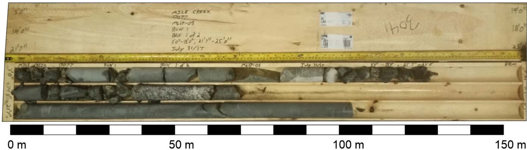
Core Photo 3: Borehole ML17-05 Rockfill and Run 1 (0.9 m to 5.5 m and 6.6 m to 7.6 m)
