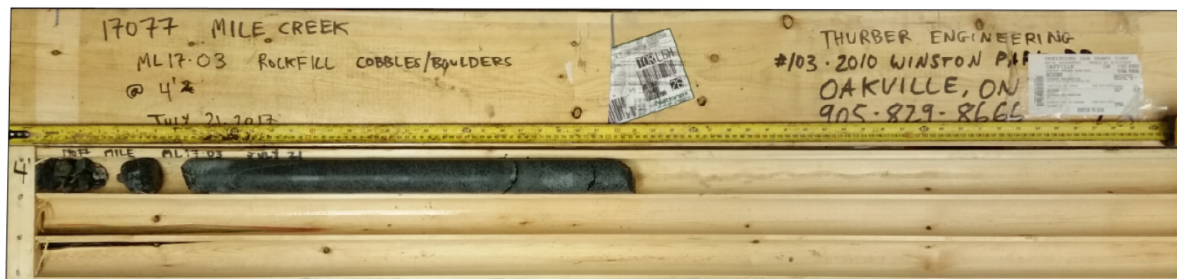
Core Photo 1: Borehole ML17-02 Run 2 to Run 3 (9.0 m to 10.6 m)
