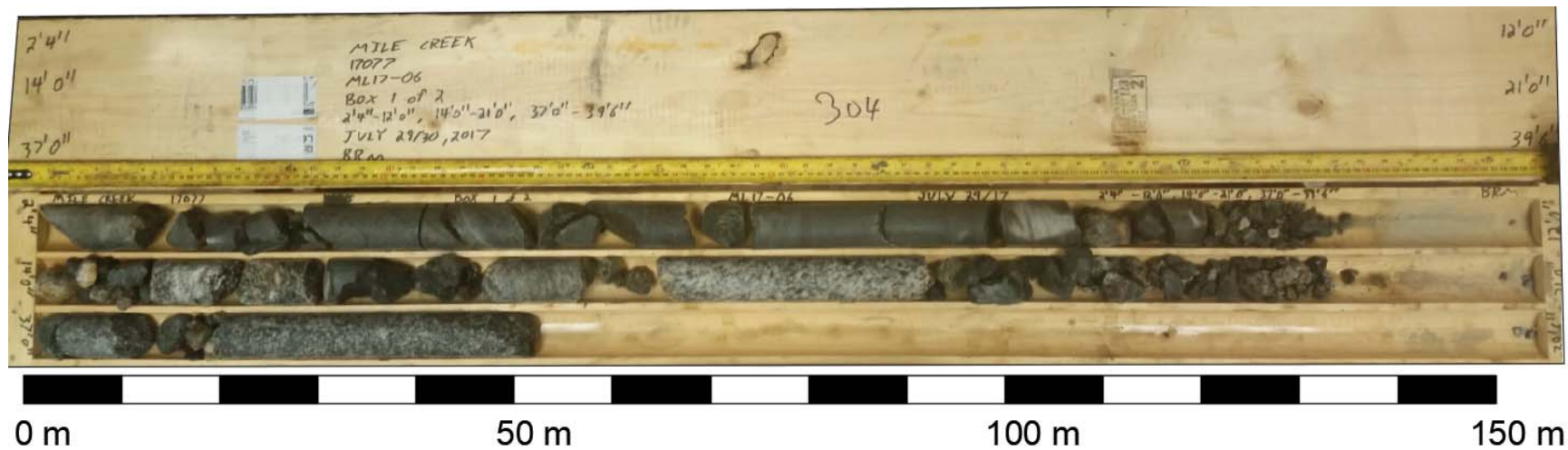
Core Photo 5: Borehole ML17-06 Rockfill and Boulders (0.7 m to 6.4 m and 11.3 m to 12.0 m)
