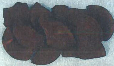
Slake Durability Test Sample (before test and after test): SL-3
