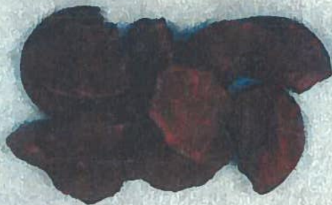
Slake Durability Test Sample (before test and after test): SL-2
