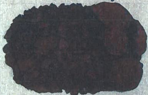
Slake Durability Test Sample (before test and after test): SL-2
