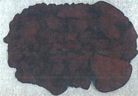
Slake Durability Test Sample (before test and after test): SL-3
