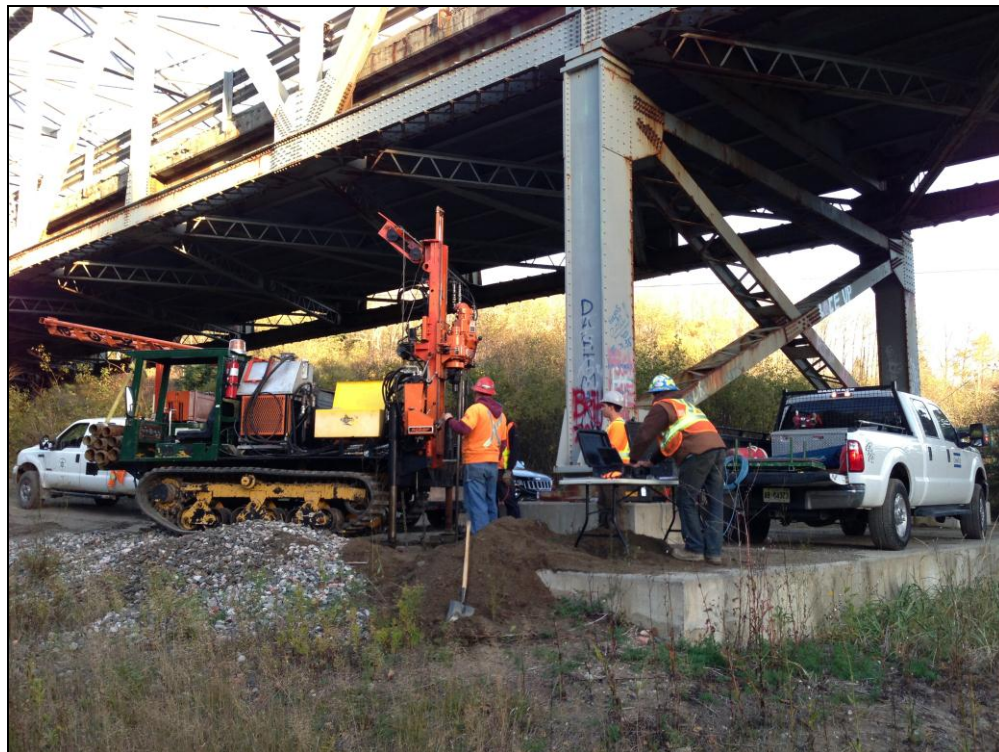
Photograph C6 – Drill Rig Set-up for Piezocone Penetration Testing, Pile E-16
