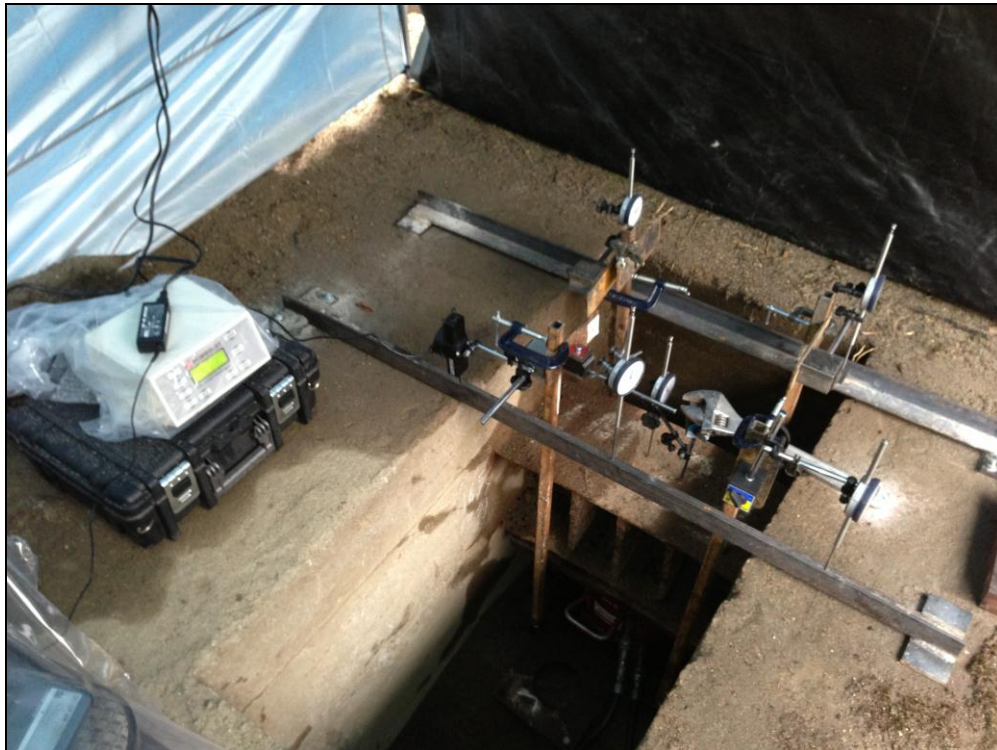
Photograph C3 – Pile Load Test Set-up at Pile E-2, West Pier
