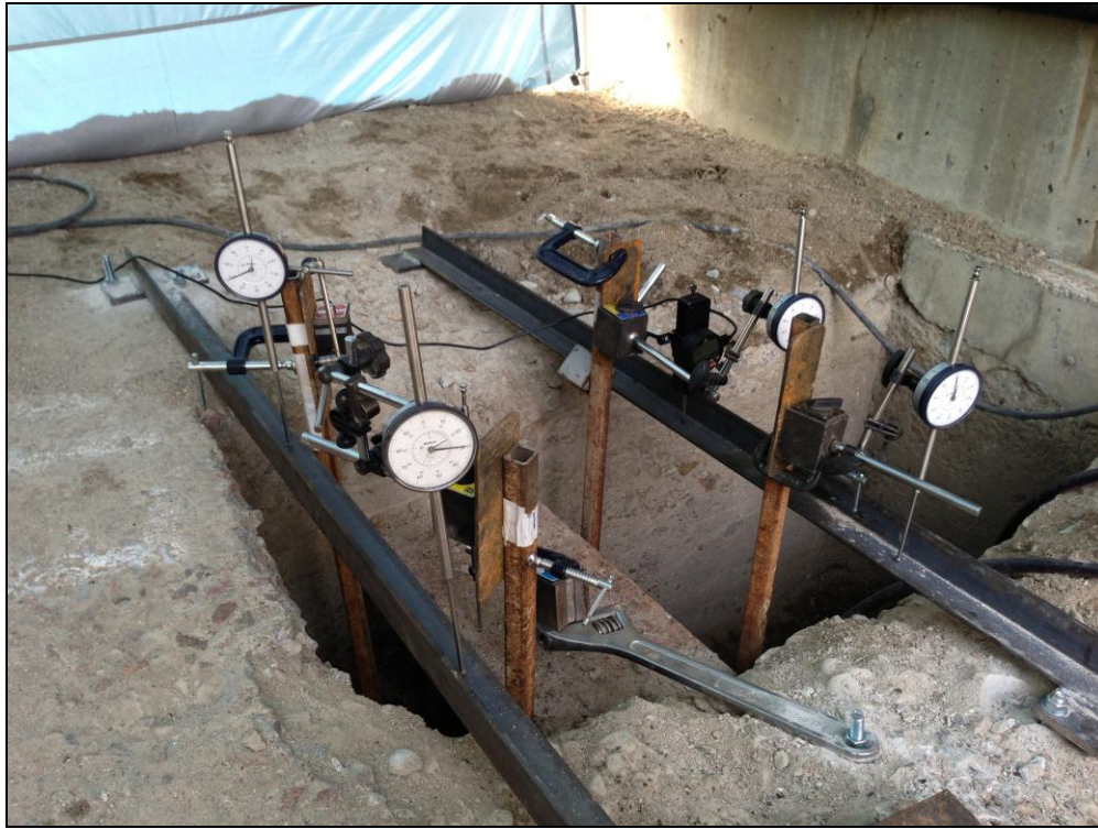
Photograph C2 – Pile Load Test Set-up at Pile E-16, East Pier
