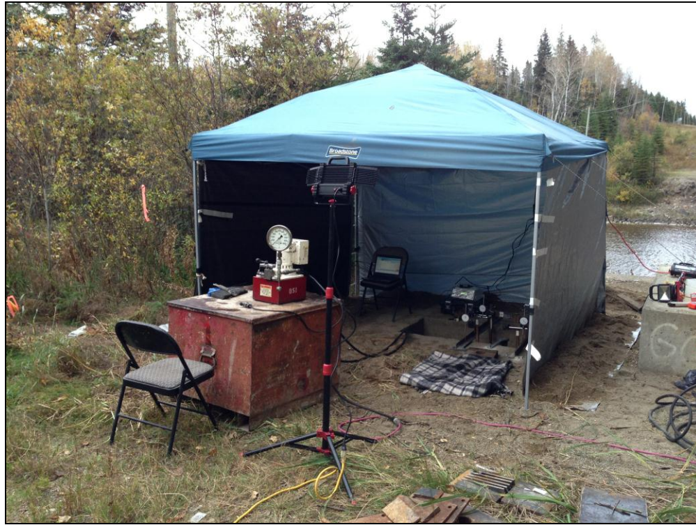
Photograph C4 – Shelter Set-up for Pile Load Test at Pier E-2
