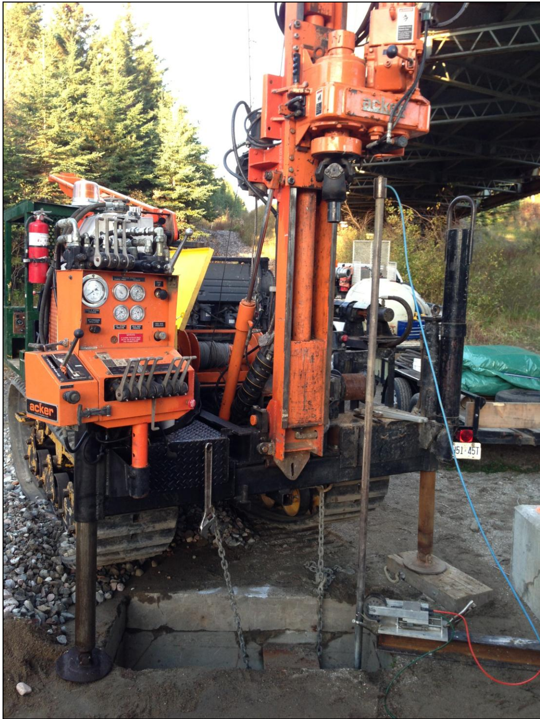
Photograph C7 – Piezocone Testing at Pile E-16
