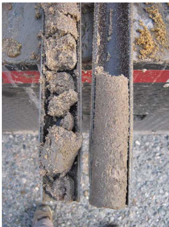
Photograph 8: View of split spoon soil sample from MMM11-04 (Nov.2, 2011).
