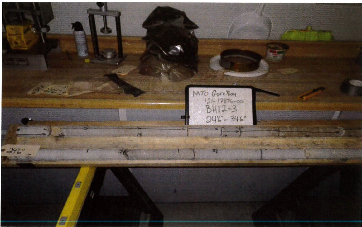
Photograph 4: BH12-3 Rock Core (7.35 m to 10.35 m).
