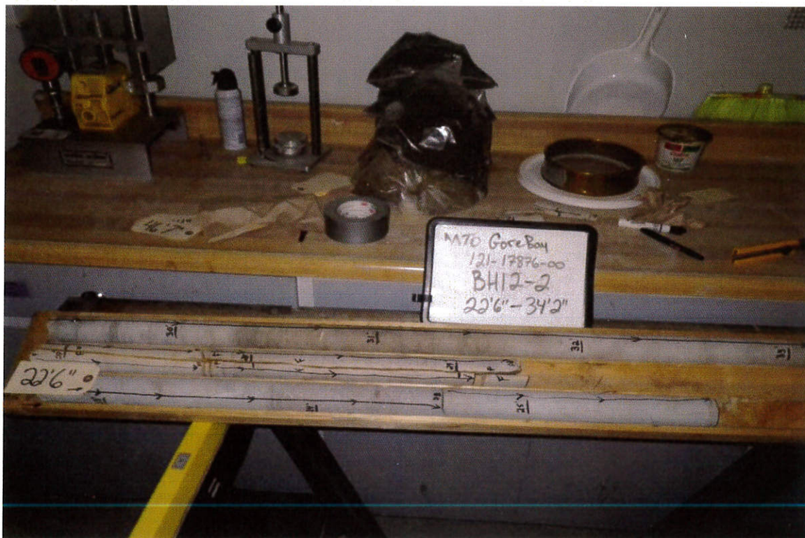
Photograph 2: BH12-2 Rock Core (6.75 m to 10.25 m).
