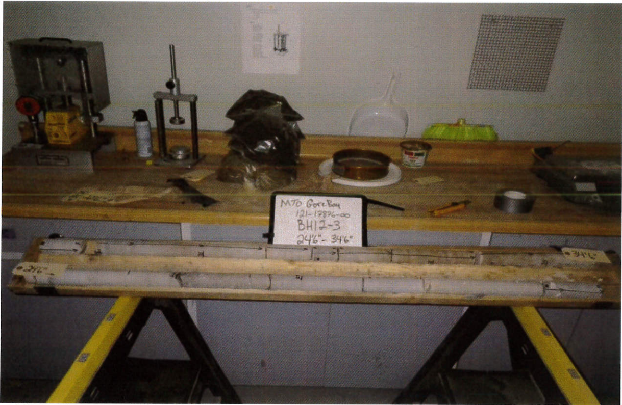
Photograph 3: BH12-3 Rock Core (7.35 m to 10.35 m).
