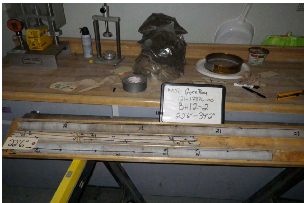
Photograph 2: BH12-2 Rock Core (6.75 m to 10.25 m).
