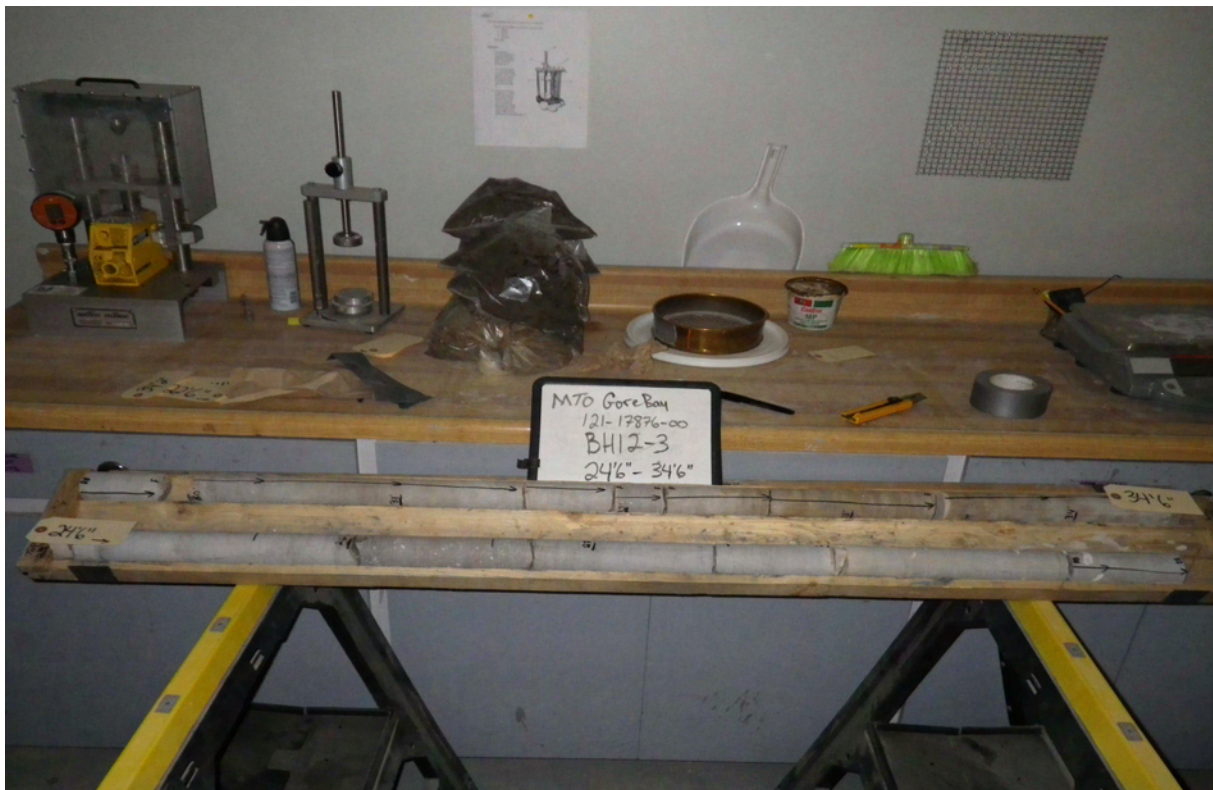
Photograph 3: BH12-3 Rock Core (7.35 m to 10.35 m).
