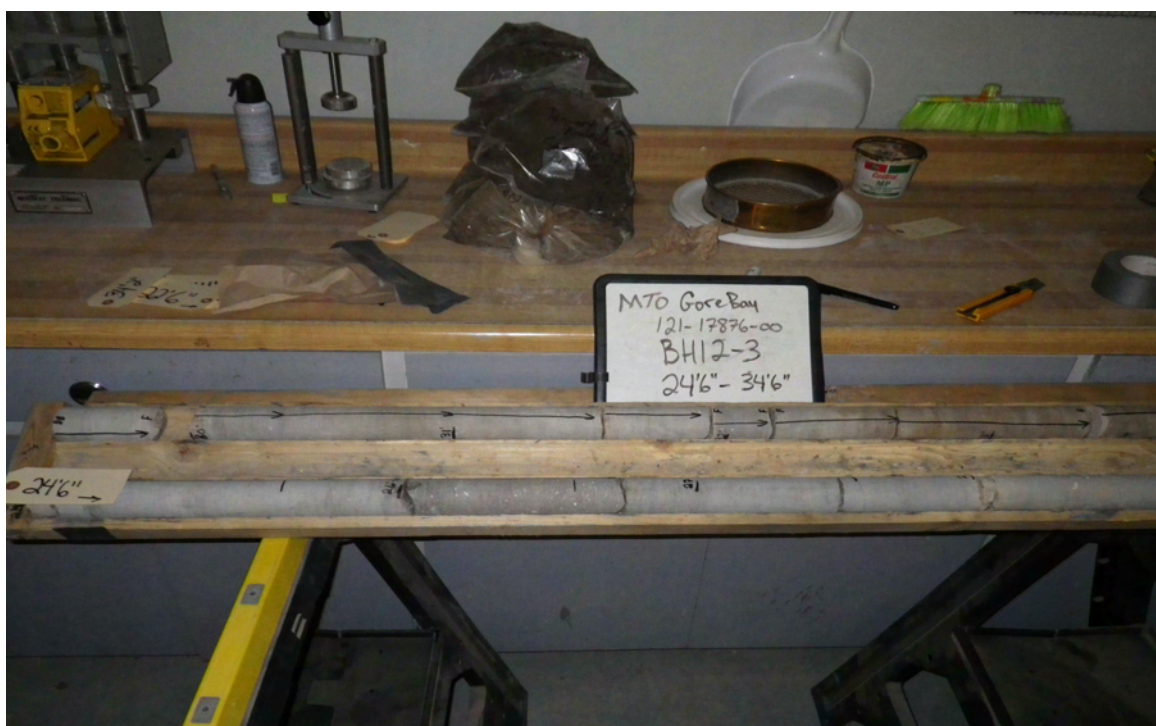
Photograph 4: BH12-3 Rock Core (7.35 m to 10.35 m).
