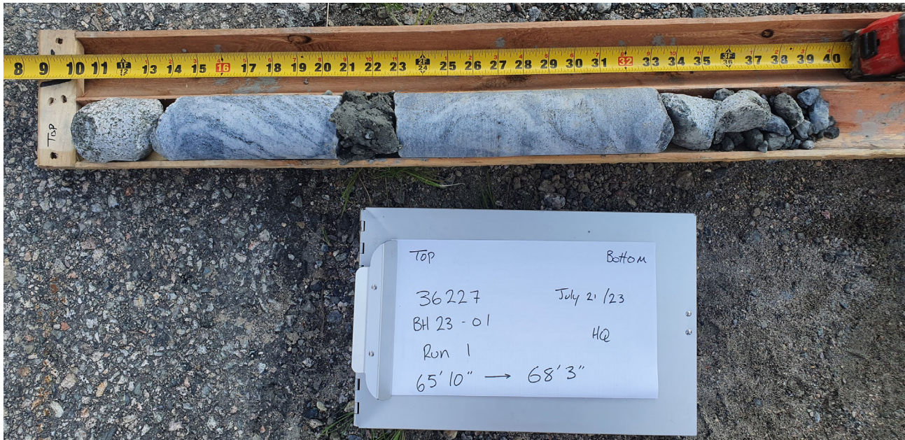
Photograph #8 – Cobbles and gravel recovered from Run 1 of Borehole 23-01.
