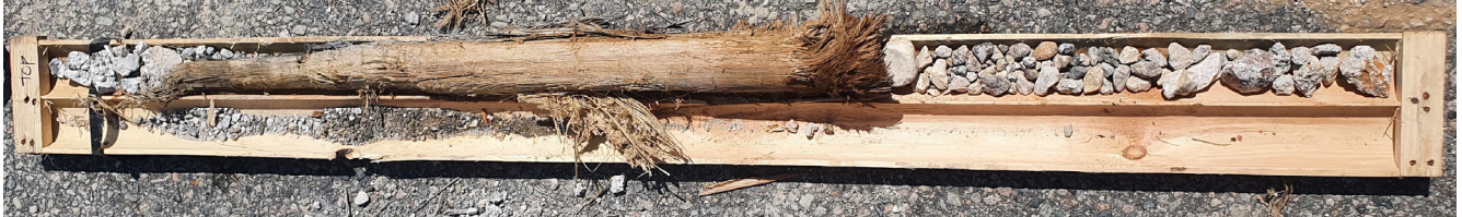
Photograph #9 – Cored wood and gravel recovered from Borehole 23-03.
