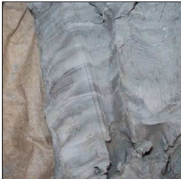
Photo 5.1 – Thinned wall tube sample showing varved clay
