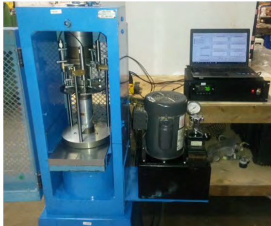
Figure 1: Forney loading frame setup for UCS testing.
