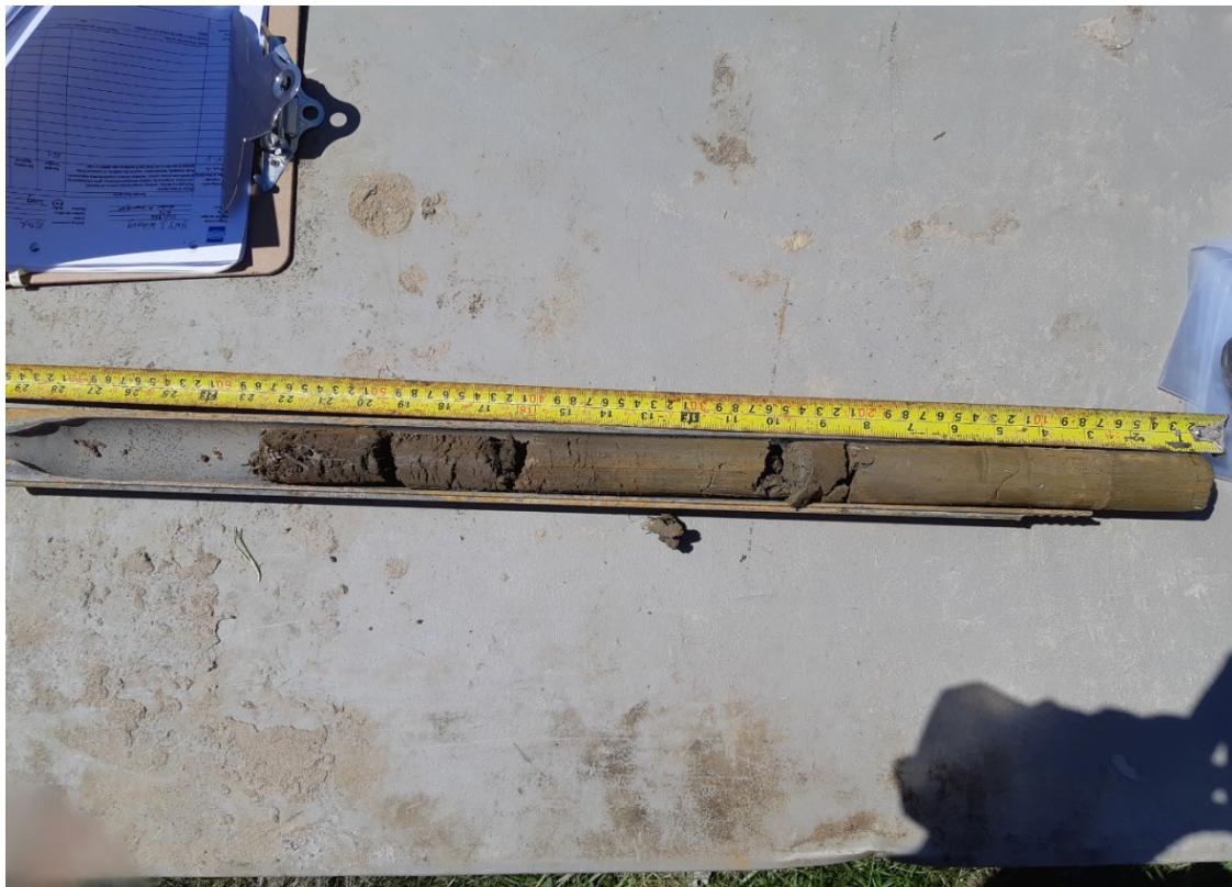
Photo 2 – A Sample of Silty Clay at BH-20-02 – Culvert No. 06X-420/C0
