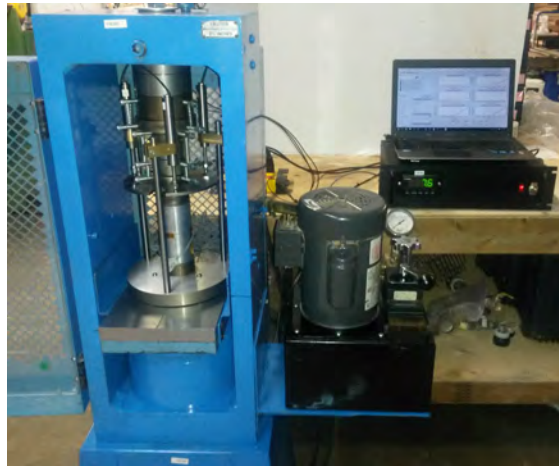
Figure 1: Forney loading frame setup for UCS testing.
