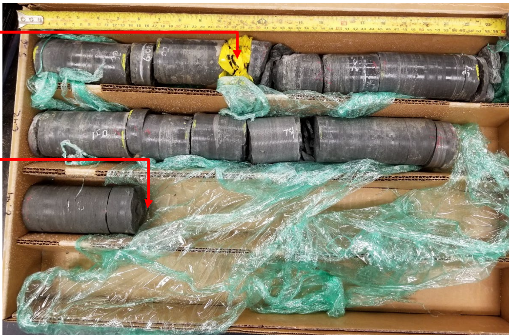
Borehole 21-01: Bedrock cored between depths of about 3.54 m to 7.11 m
