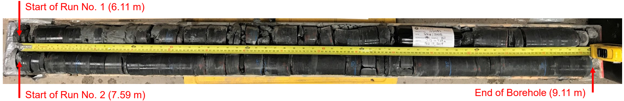
OPB-1 Rock Core: 6.11 m to 9.11 m depth
