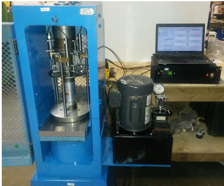
Figure 1: Forney loading frame setup for UCS testing.
