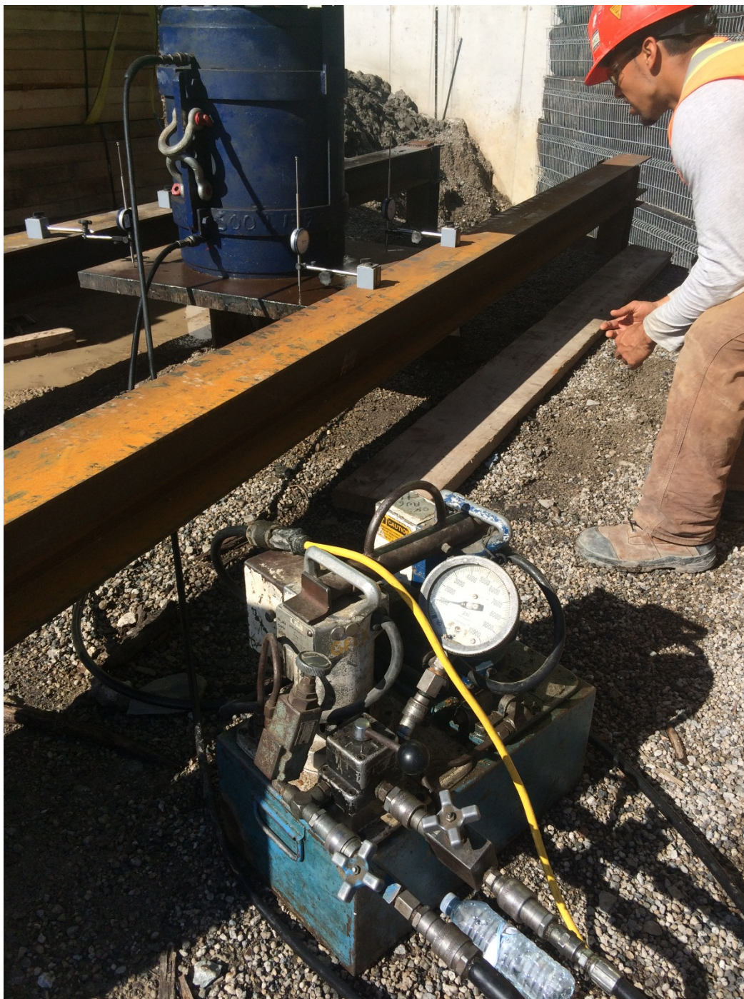
Photograph 6: Static load testing underway, hydraulic pressure gauge in foreground
