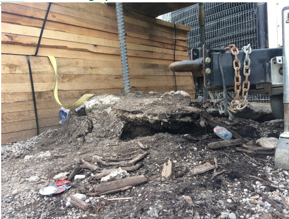
Photograph 7: Reaction Caisson heave / failure during load test (north side)
