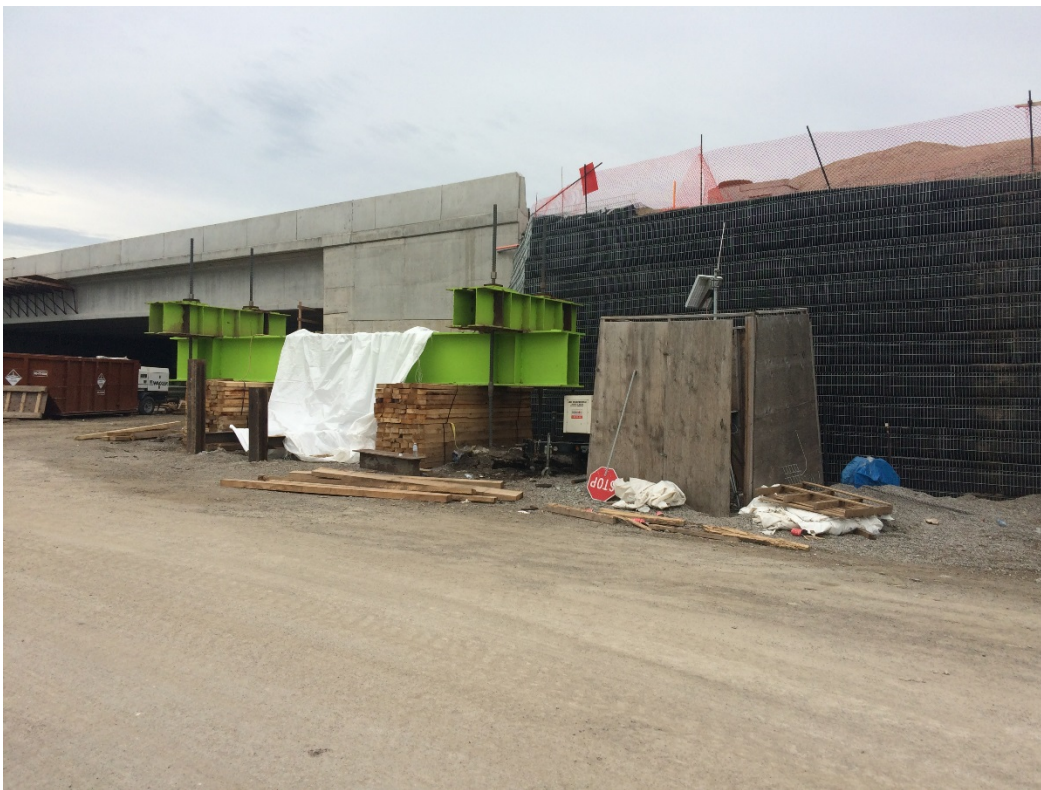
Photograph 1: Static load test reaction frame set-up
