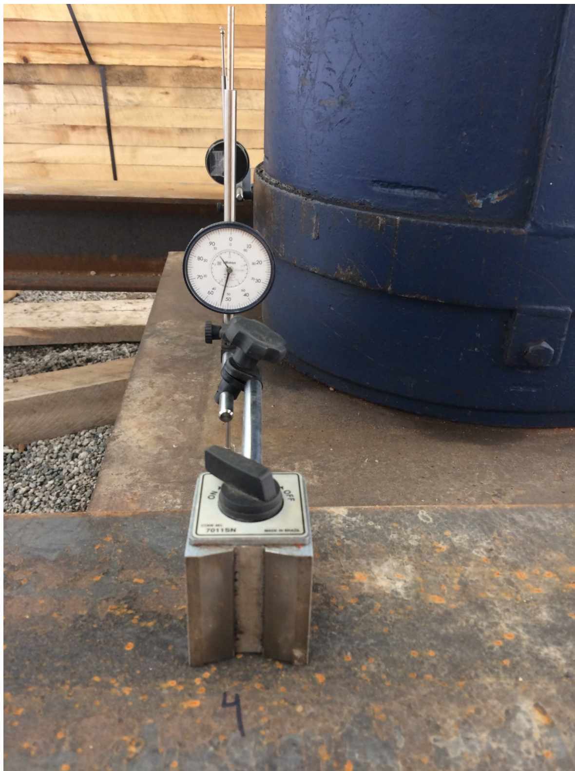
Photograph 3: Dial gauge on independent reference beam
