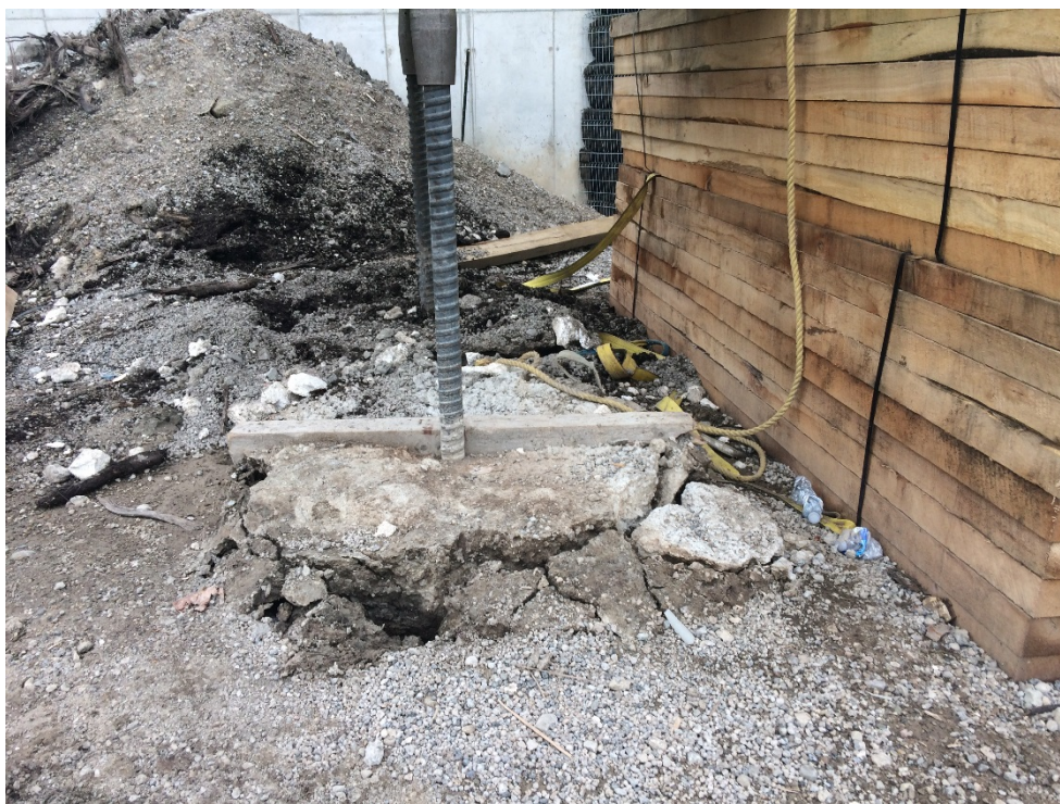
Photograph 8: Reaction Caisson heave / failure during test (south side)
