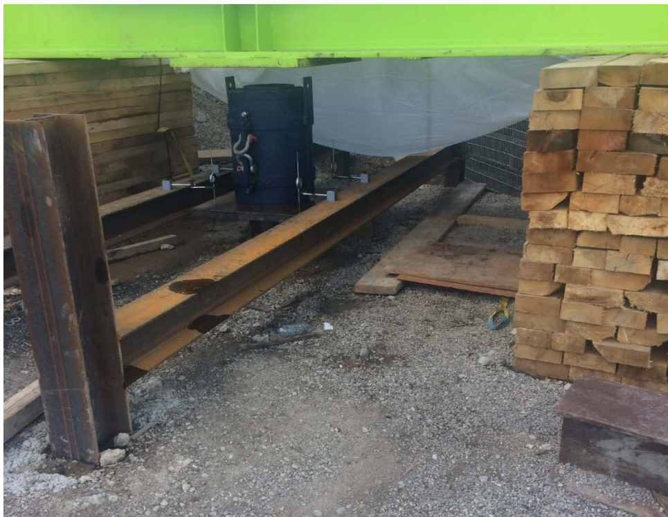
Photograph 4: Hydraulic jack and dial gauge set-up
