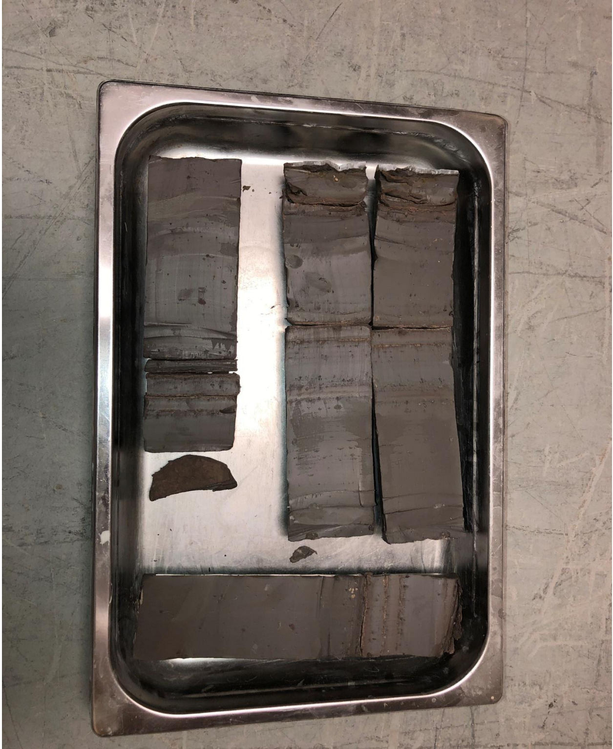
Photograph 4: Soil sample extracted at Glendale Avenue and QEW Interchange, the varved clay structure observed in clay material collected in borehole RSS2.
