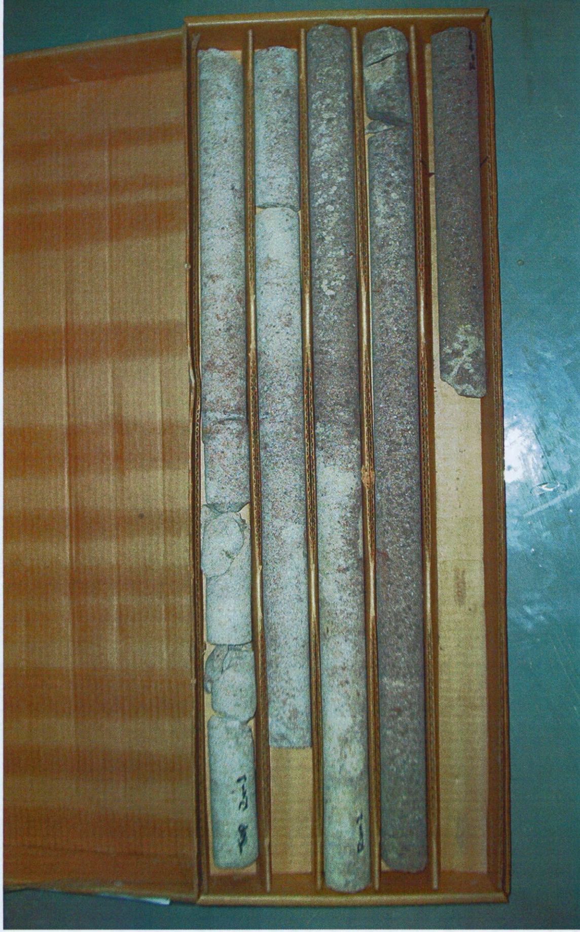
PHOTOGRAPH OF BEDROCK CORE Borehole 15+975, 17m Lt, Quartzite Bedrock
