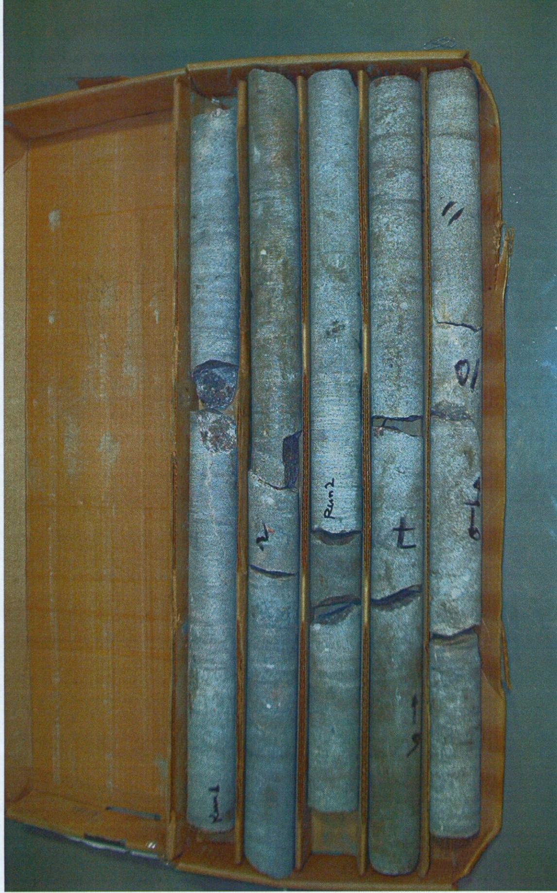
PHOTOGRAPH OF BEDROCK CORE Borehole 15+730, 20m Lt, Quartzite Bedrock
